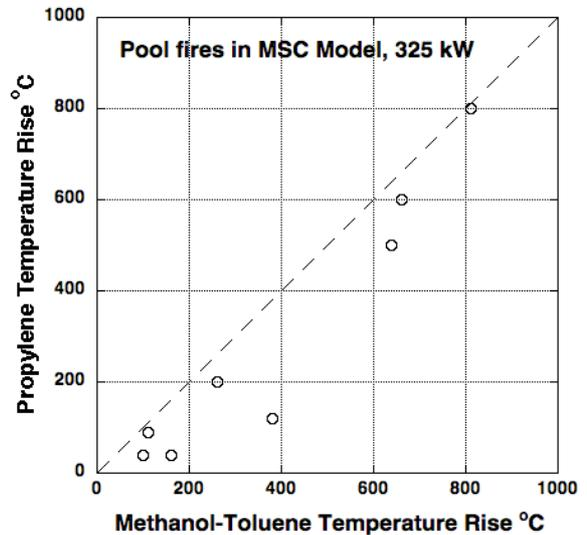
Fig. 8: Comparison of temperature in the model as simulated by propylene gas and methanol-toluene liquid at 325 kW
