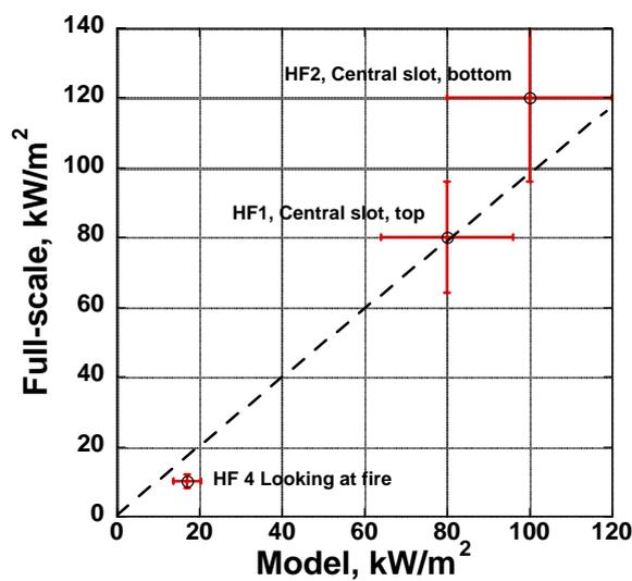
Fig. 7: Comparison of heat flux in full-scale and model
