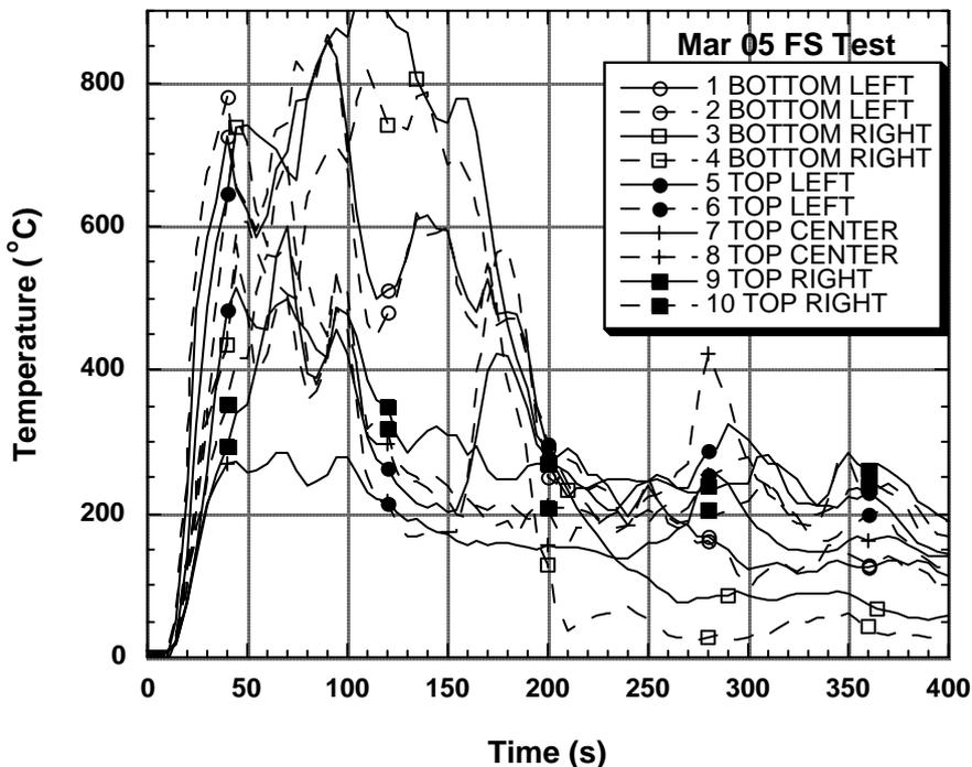
Fig. 16: Temperature results in the full-scale MSC 914 test with 2 TF18 nozzles
