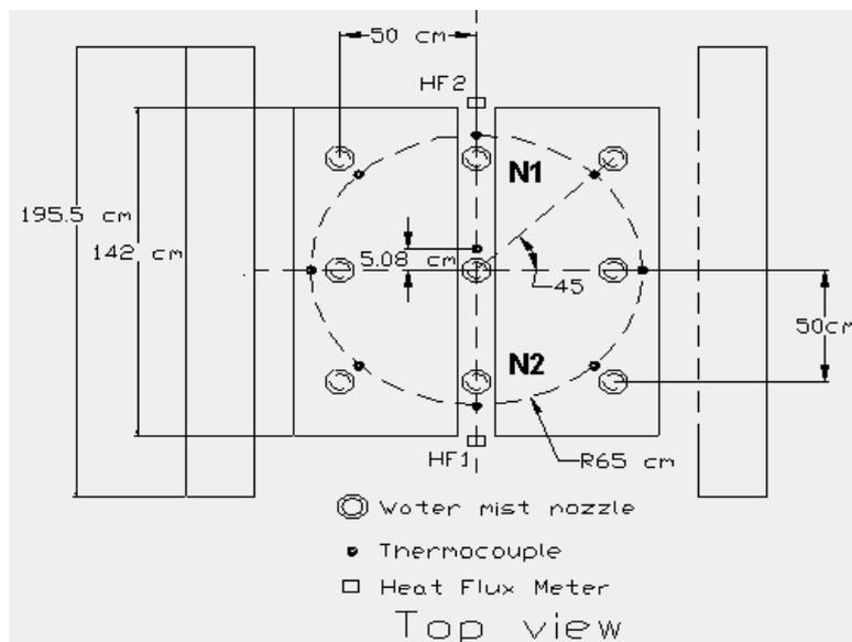
**Fig. 10: Nozzle and instrumentation in scaled suppression tests**
