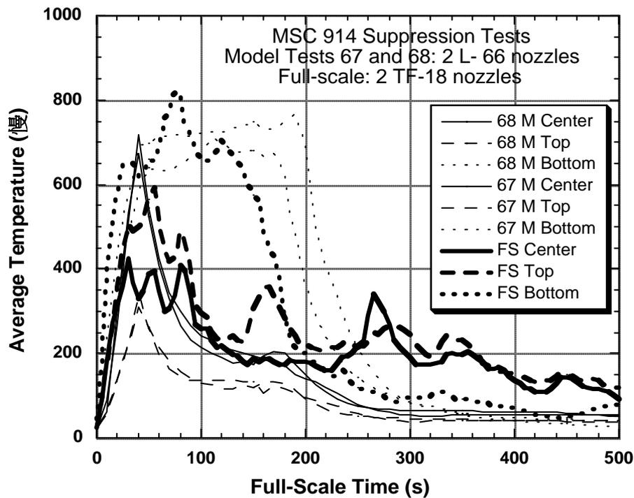
Fig. 17: A comparison between model and full-scale temperatures
