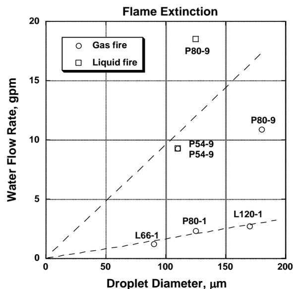
**Fig. 12: Water flow rate for suppression in the scaled tests (1 gpm = 63 mL·s<sup>-1</sup>)**
