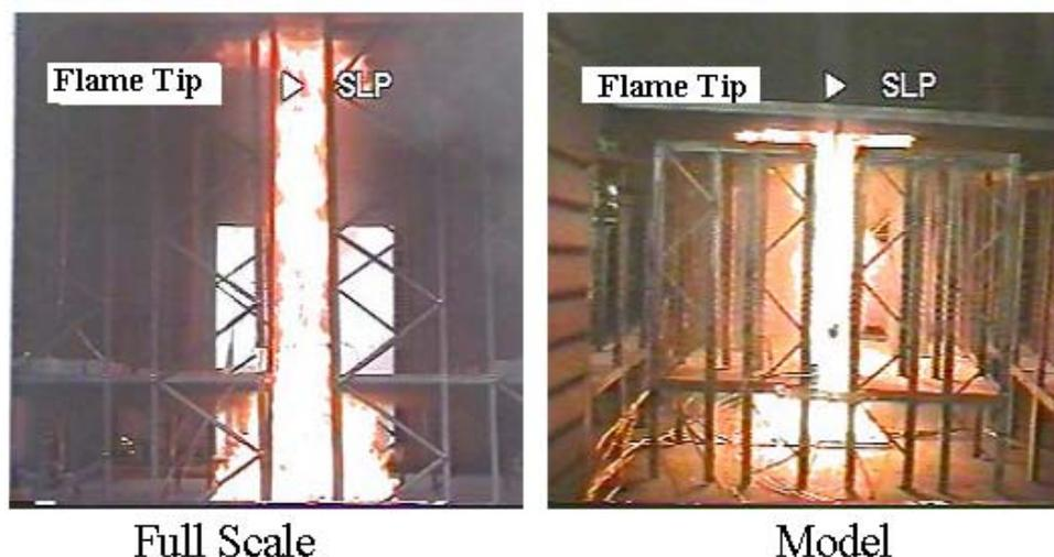
Fig. 4: Comparison of flame shape in full-scale and model
