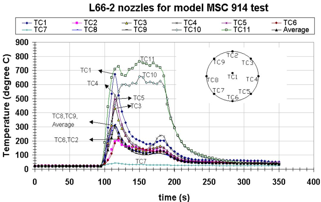
Fig. 15: Ceiling and underside temperatures for the model test with 2 L66 nozzles
