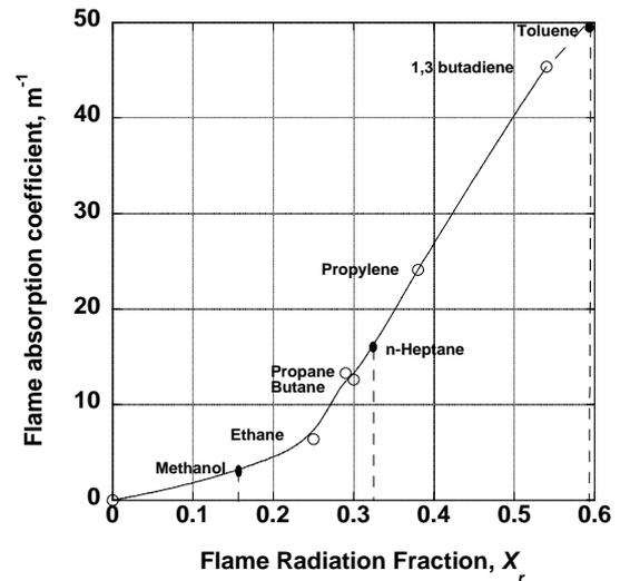
**Fig. 3: Correlation for absorption coefficient and radiative fraction**
