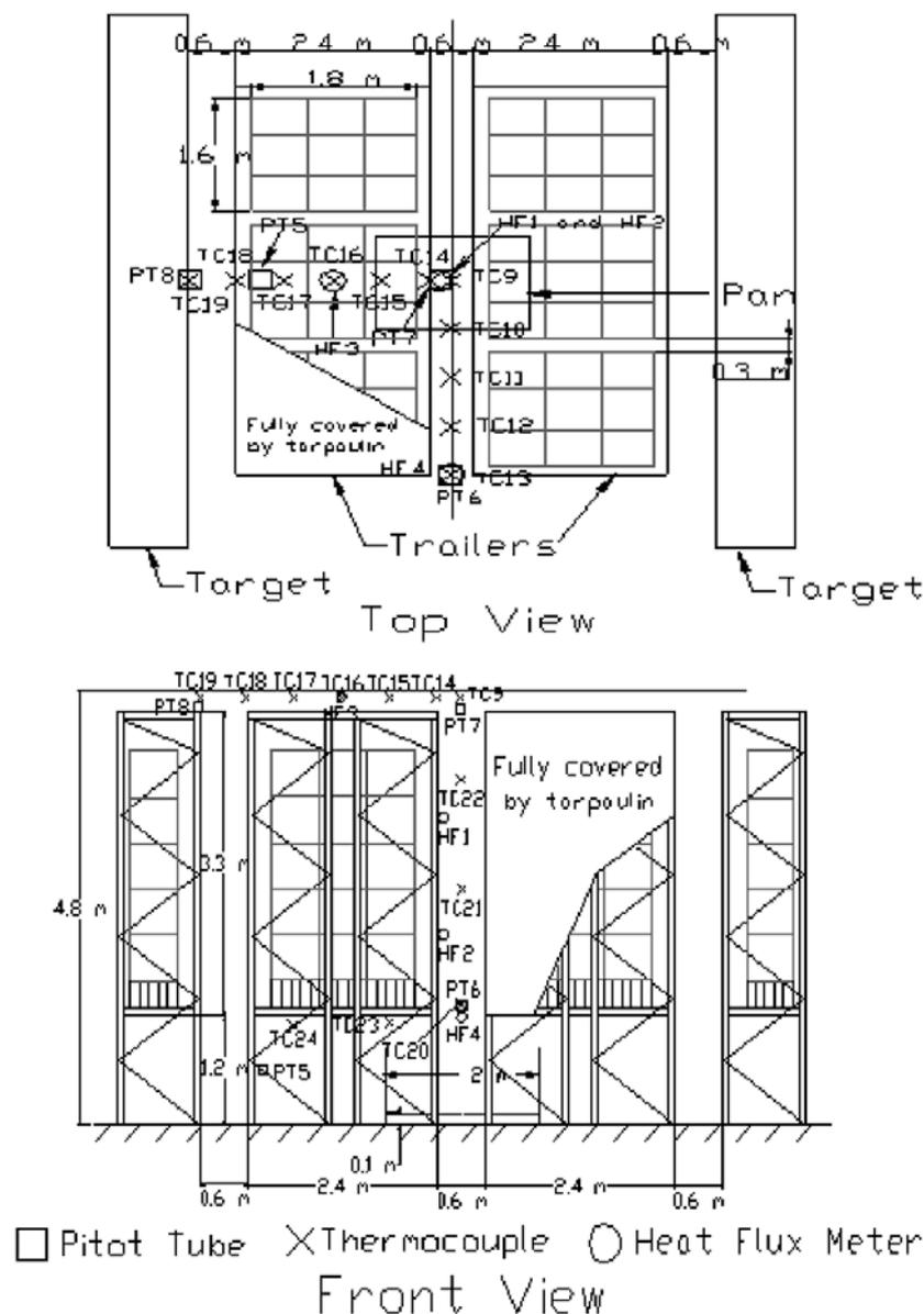
Fig. 1: MSC 914 test layout
