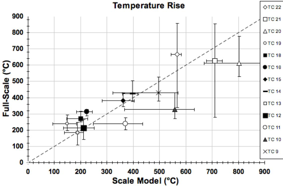
Fig. 6: Comparison of peak temperature rise for all thermocouples
