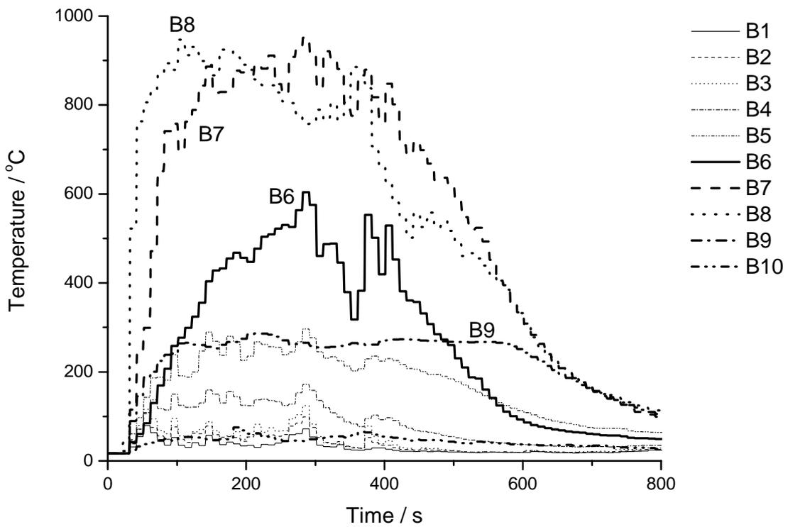
Fig. 8: Temperature profile of thermocouple tree B
