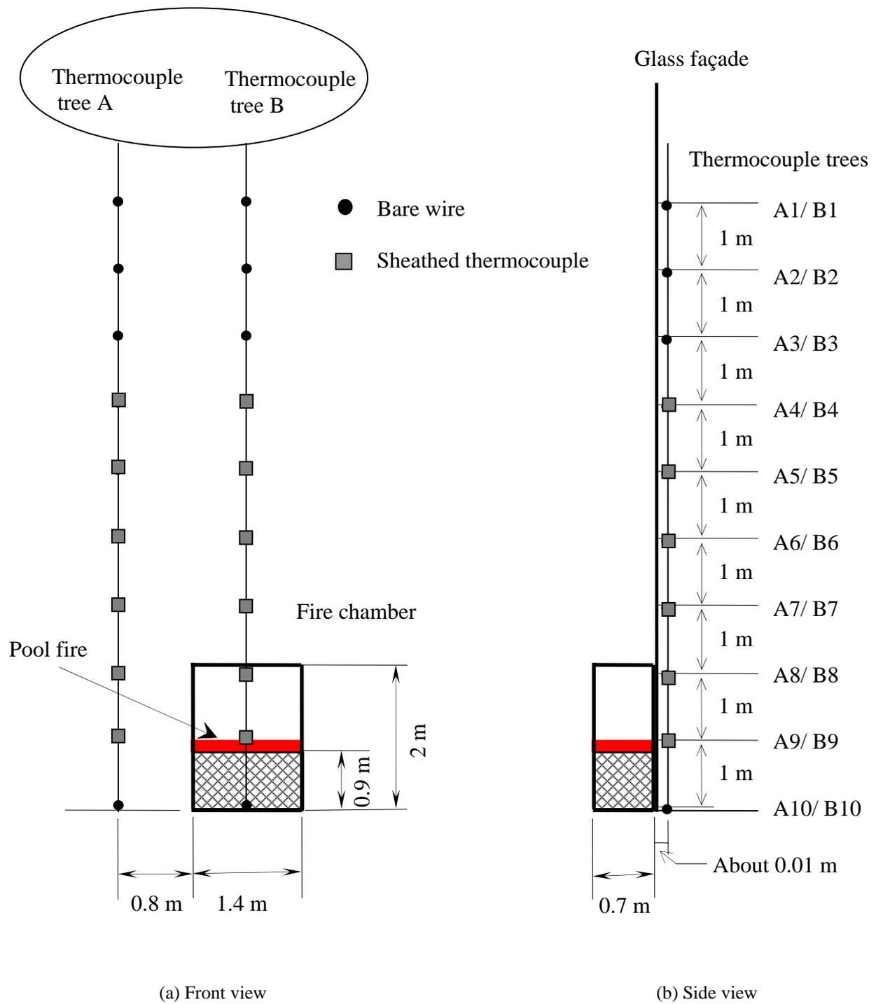
Fig. 6: Location of thermocouples
