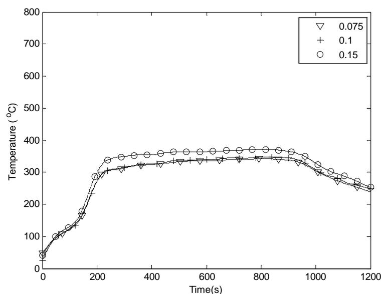
Fig. 4: Temperature profiles at thermocouple 2 for varying grid sizes
