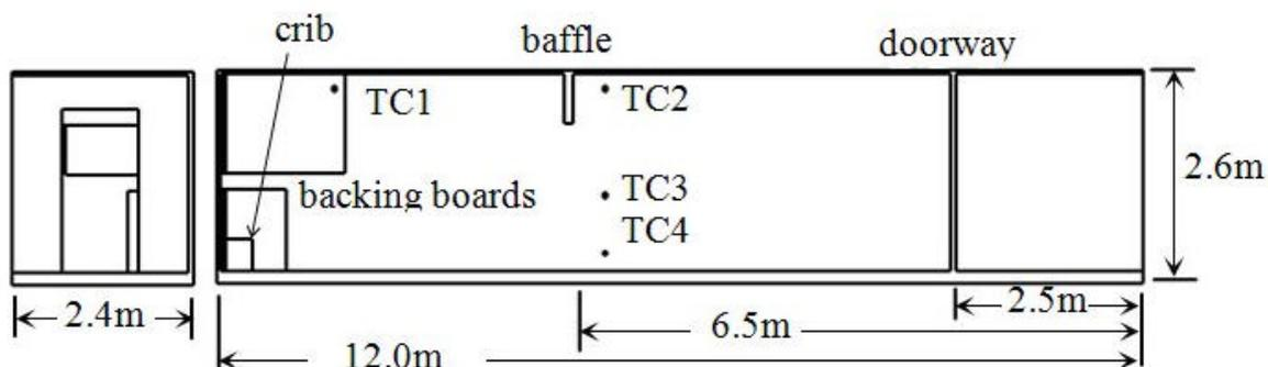
**Fig. 2: CFBT demonstration cell**
