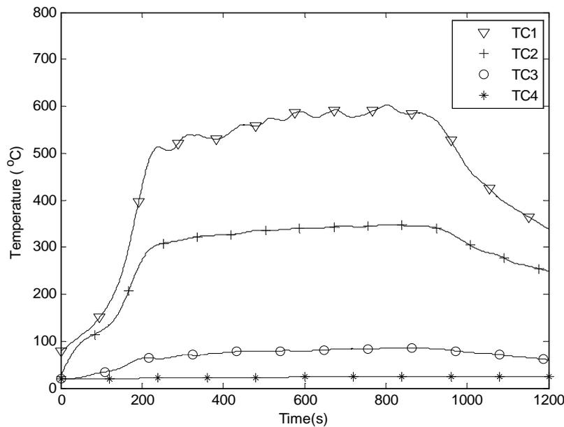
**Fig. 9: FDS temperature profiles of the demonstration cell without the baffle at four thermocouple locations**
