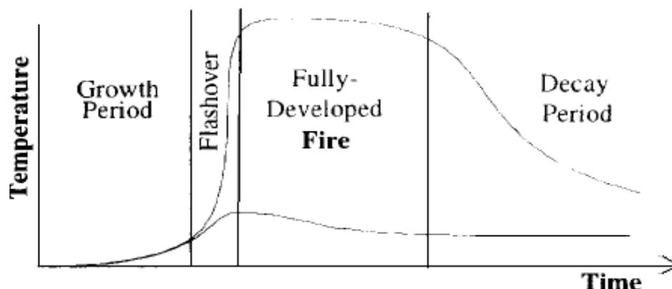
Fig. 1: Stages in a compartment fire temperature history [1]
