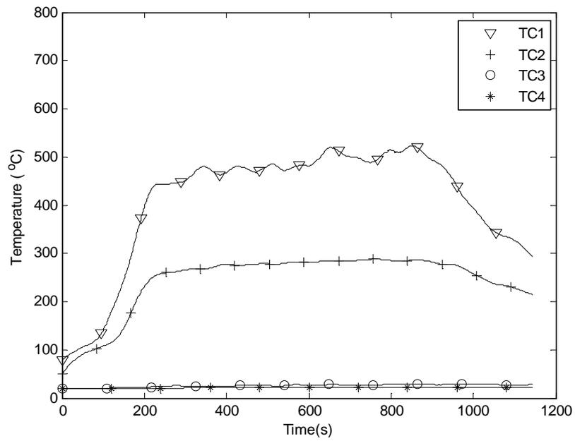
Fig. 7: FDS temperature profiles of the demonstration cell with vent open at four thermocouple locations
