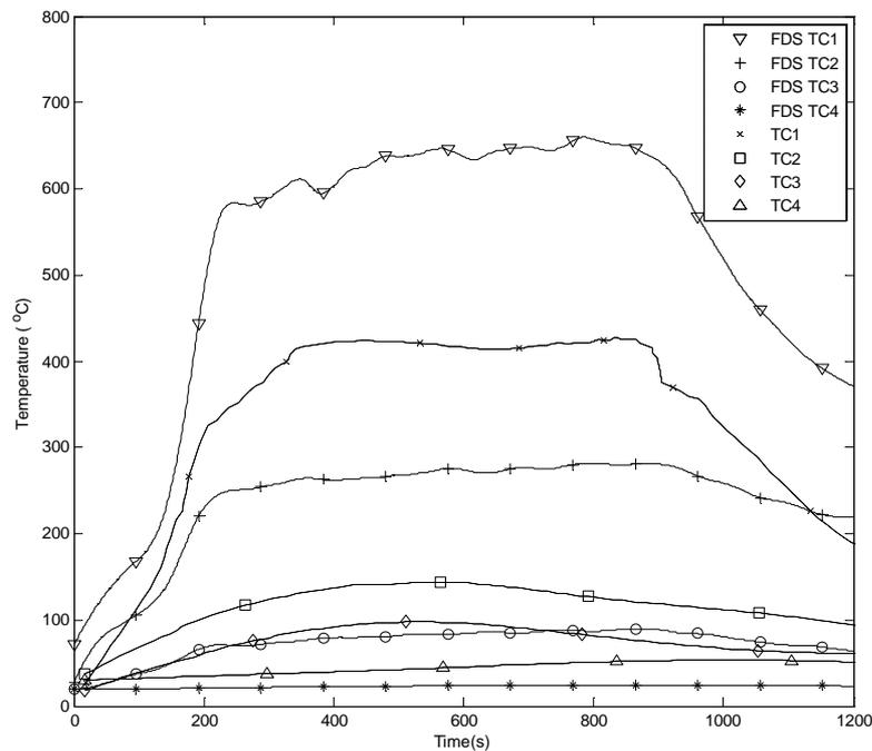
**Fig. 6: FDS temperature profiles at four thermocouple locations**
