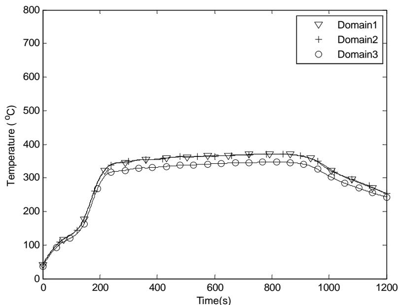
Fig. 5: Temperature profiles at thermocouple 2 for varying domain sizes
