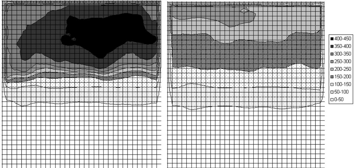
(a) On fire side of the baffle
