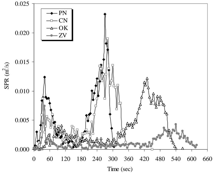
Fig. 4: SPR curves of native wood species at 50 kWm<sup>-2</sup> external heat flux (PN: Pitch Pine, CN: Chestnut Tree, OK: Oak, ZV: Zelkova)
