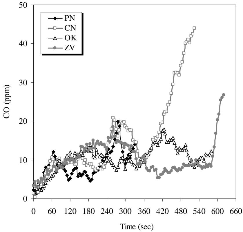
Fig. 6: CO production curves of native wood species at  $50 \text{ kWm}^{-2}$  external heat flux (PN: Pitch Pine, CN: Chestnut Tree, OK: Oak, ZV: Zelkova)
