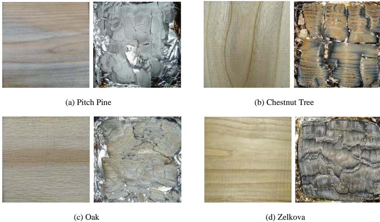
**Fig. 3: Native wood before burning and the residues of native wood after combustion**
