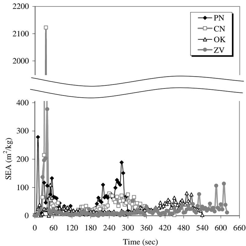
Fig. 5: SEA curves of native wood species at 50 kWm<sup>-2</sup> external heat flux (PN: Pitch Pine, CN: Chestnut Tree, OK: Oak, ZV: Zelkova)
