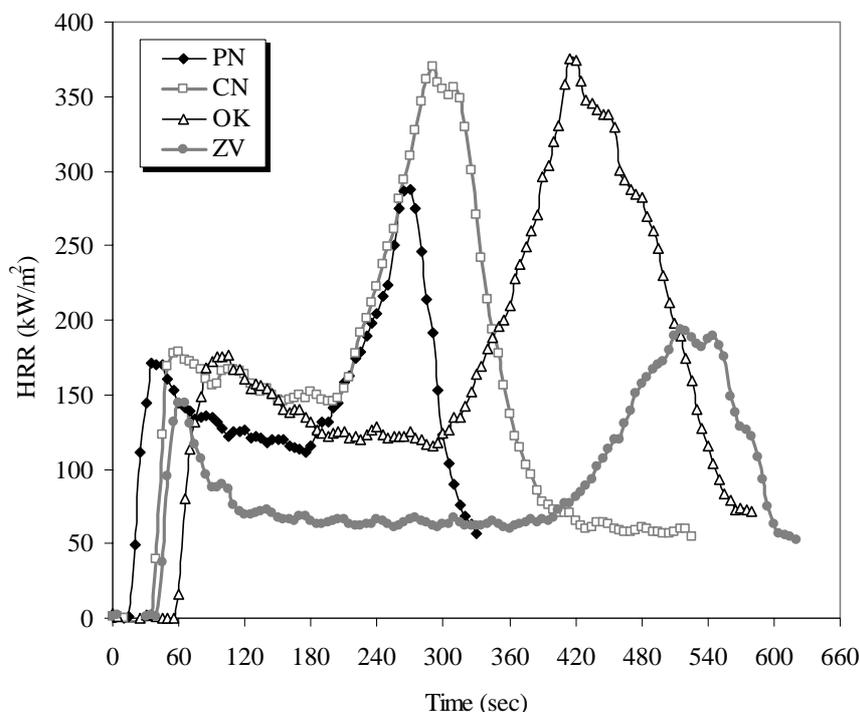
Fig. 1: HRR curves of native Korean wood species at 50 kWm<sup>-2</sup> external heat flux (PN: Pitch Pine, CN: Chestnut Tree, OK: Oak, ZV: Zelkova)
