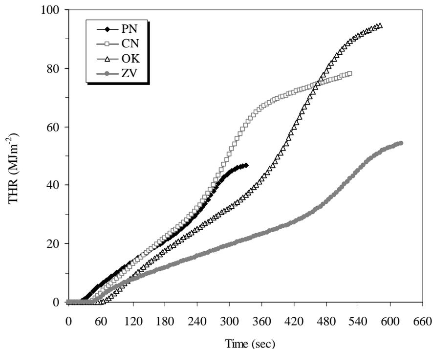
**Fig. 2: THR curves of native wood species at 50 kWm<sup>-2</sup> external heat flux (PN: Pitch Pine, CN: Chestnut Tree, OK: Oak, ZV: Zelkova)**
