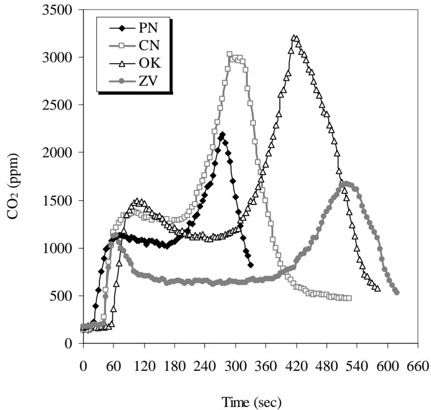
Fig. 7: CO<sub>2</sub> production curves of native wood species at  $50 \text{ kWm}^{-2}$  external heat flux (PN: Pitch Pine, CN: Chestnut Tree, OK: Oak, ZV: Zelkova)
