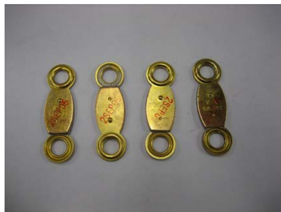
Fig. 4: The four fusible links tested on 25 January 2006
