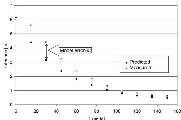
Fig. 4: Data from a fire scenario used to illustrate the variation of the error within a scenario
