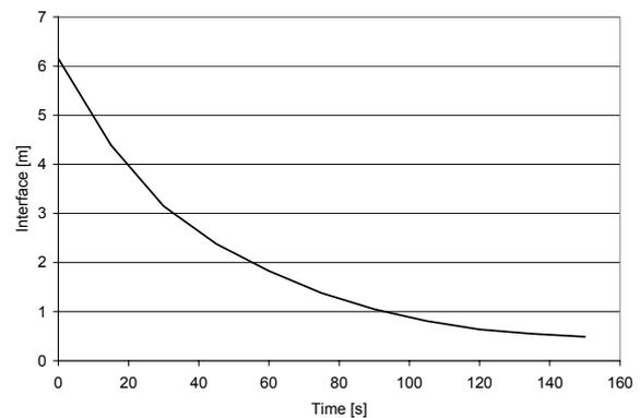
Fig. 2: Interface,  $z$ , as a function of time after ignition
