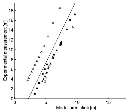
**Fig. 19: Measured interface height plotted against predicted interface height. The regression line is also shown.**
