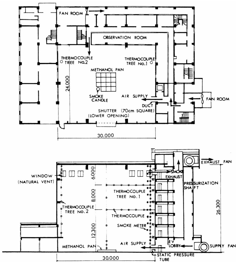
Fig. 12: Plan and section of the room where the experiments were conducted [20]
