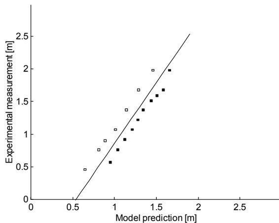
**Fig. 17: Measured interface height plotted against predicted interface height. The regression line is also shown.**
