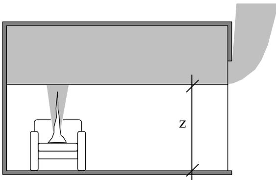
Fig. 1: Illustration of a two-zone model
