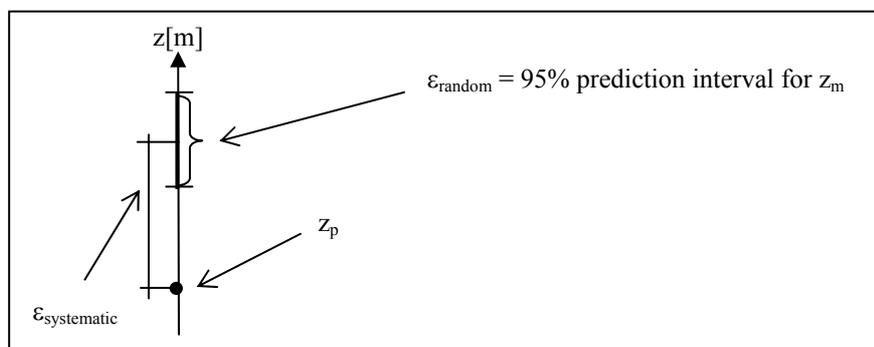
Fig. 5: Definition of the model error for a specific scenario configuration, i.e. as a combination of a random and a systematic error for each model prediction
