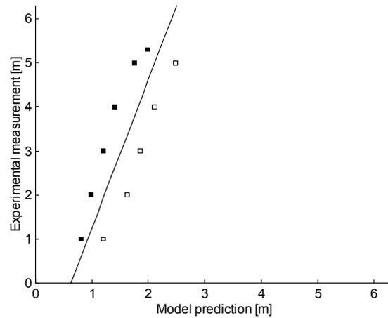
**Fig. 15: Measured interface height plotted against predicted interface height. The regression line is also shown**
