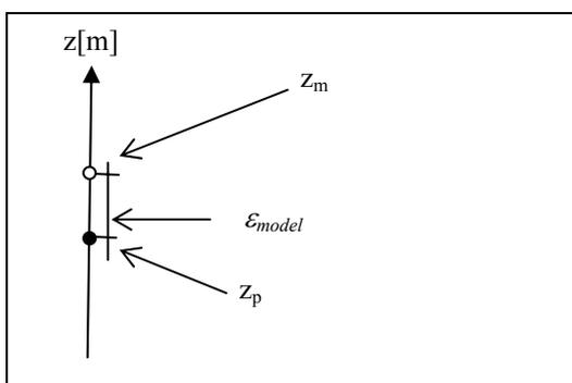
Fig. 3: Definition of the model error for a single prediction and measurement
