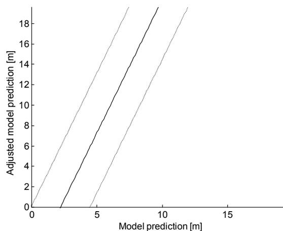
**Fig. 20: Mean estimate and 95% prediction interval for the adjusted model prediction of the interface height**
