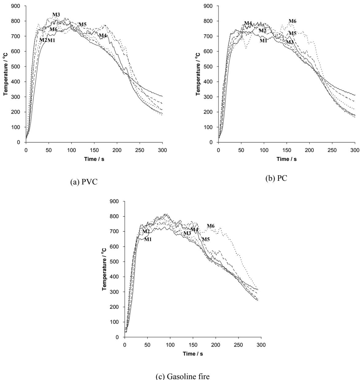
**Fig. 7: Fire plume temperature for scenario II**
