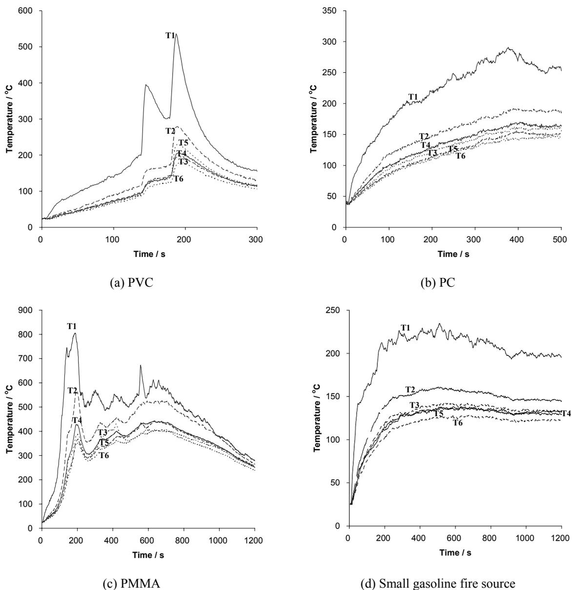
Fig. 5. Upper layer gas temperature for scenario I
