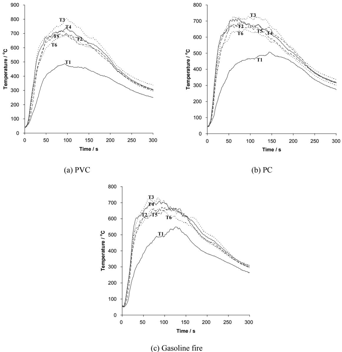
**Fig. 8: Upper layer gas temperature for scenario II**
