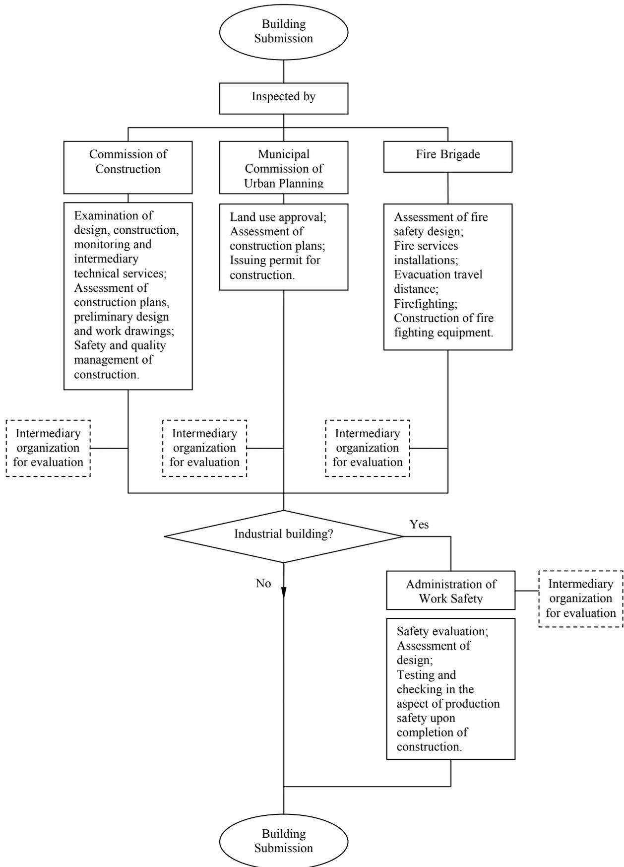
Fig. 1: Assessment and approval of building constructions
