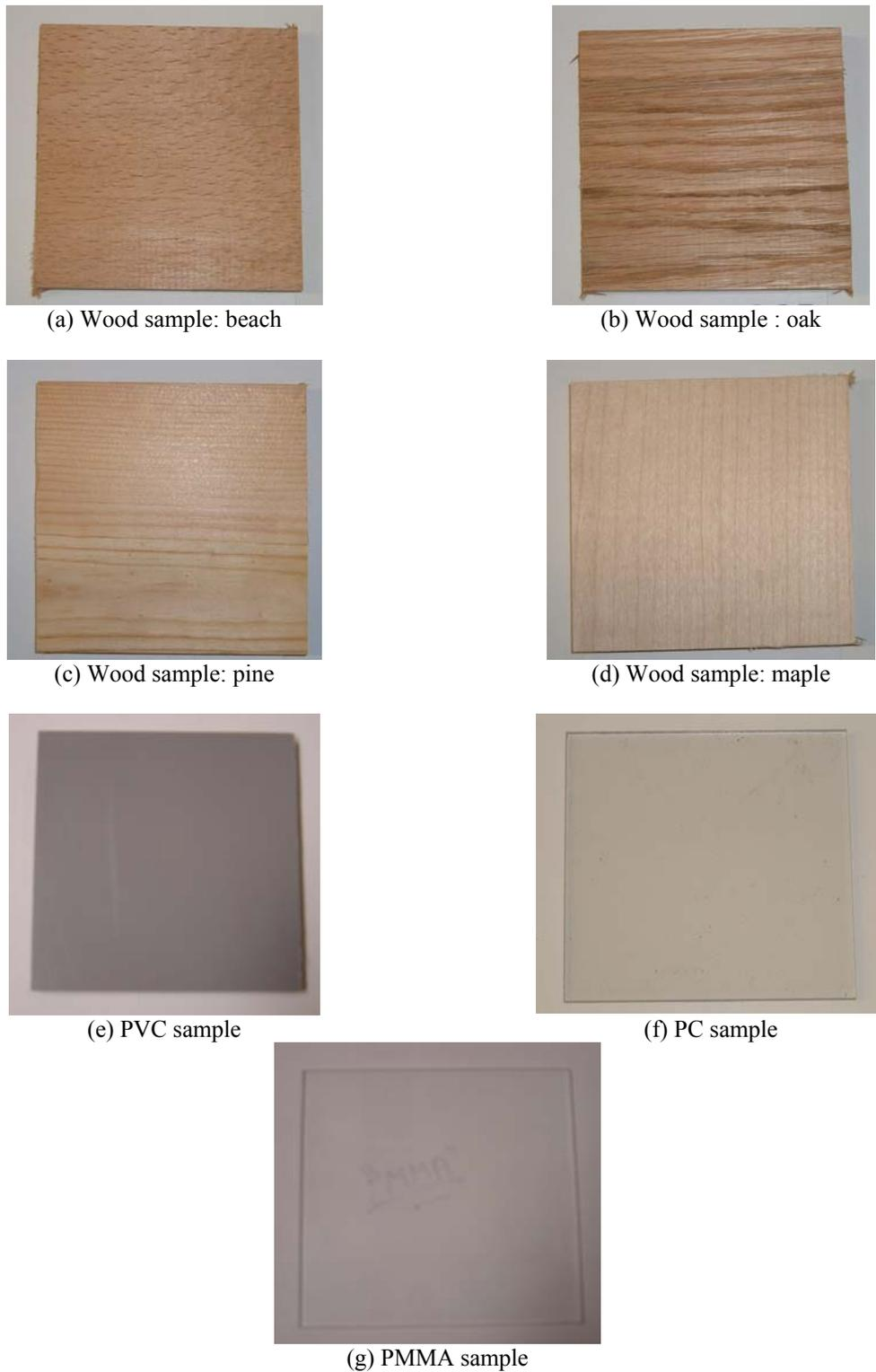
**Fig. 1: Samples tested**
