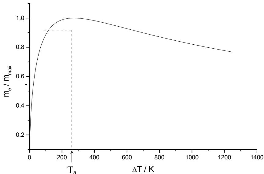
Fig. 4: Effects of the temperature on mass flow through the vent
