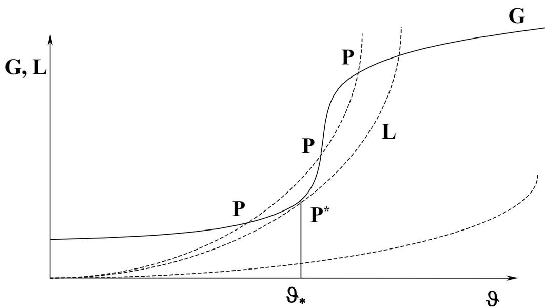
Fig. 1: Semenov's diagram for thermal explosion or flashover
