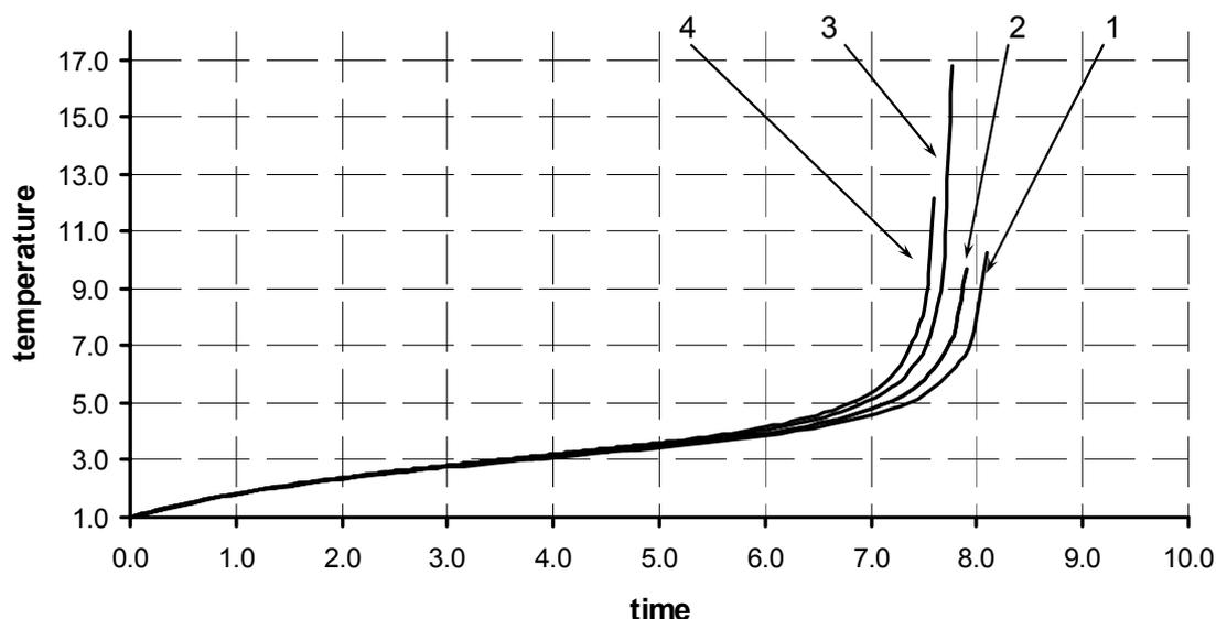
**Fig. 6: Influence of sprinkler activation temperature on flashover induction period**
