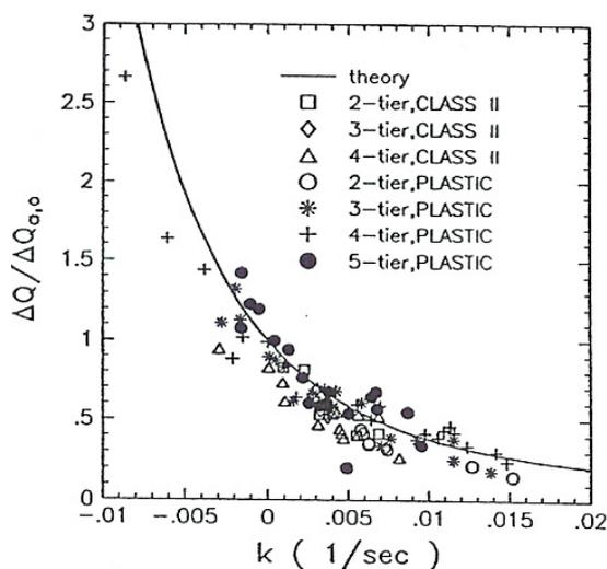
**Fig. 4: Test data by Yu et al. [9] and its correlation with the fire suppression parameter  $k$  (“extinction constant”)**
