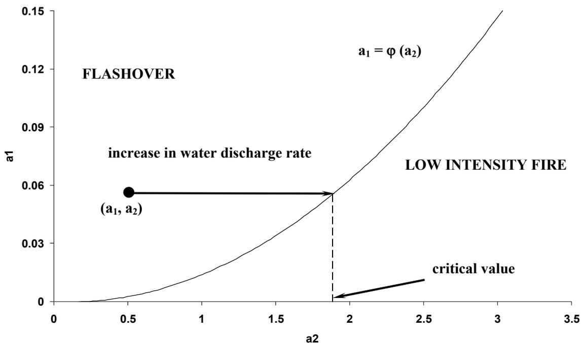
Fig. 2: Effect of heat extraction from smoke layer on critical conditions for flashover [10]
