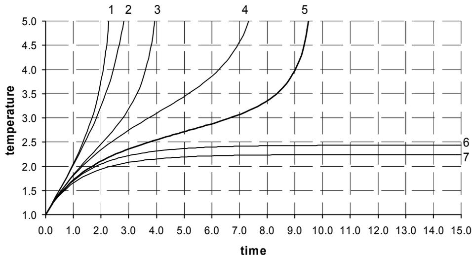
**Fig. 5: Temperature histories for original model without suppression [6] and the present model. Fire compartment conditions correspond to example considered in [6].**
