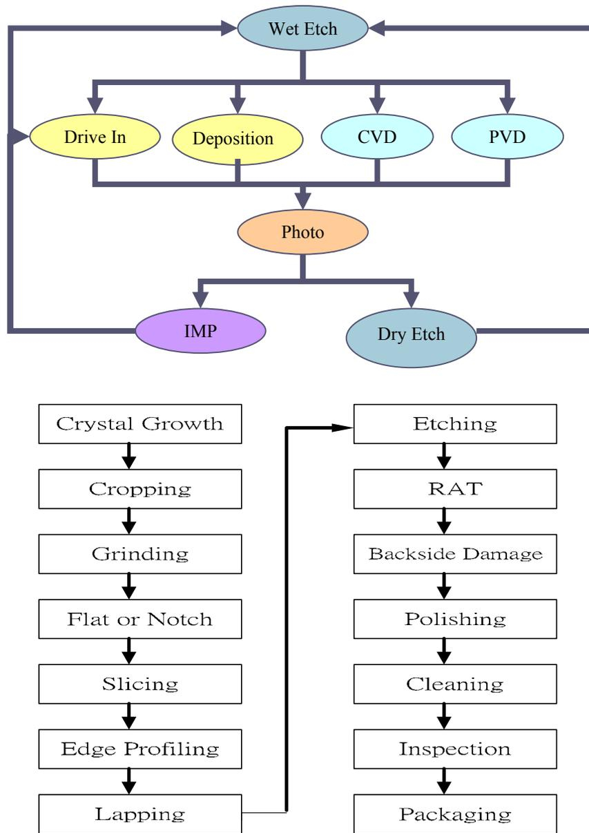
Fig. 2: Diagram of wafer manufacture
