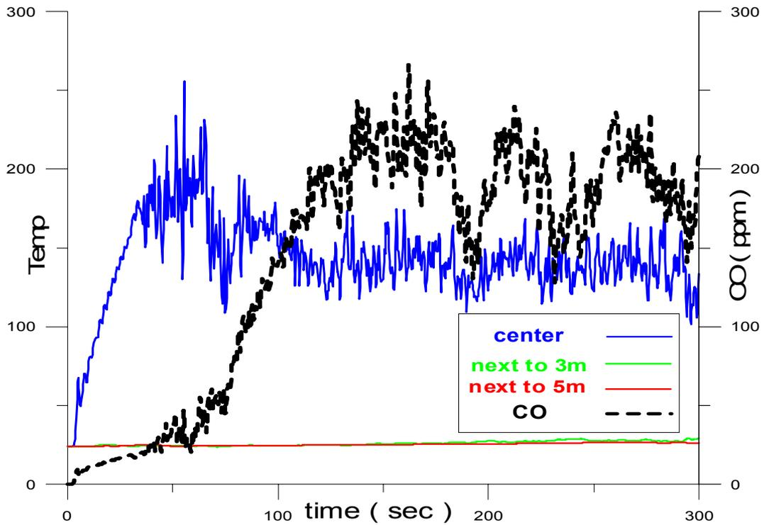
Fig. 11a: The temperature and CO concentration measured variation at 1.8 m (scenario 4)
