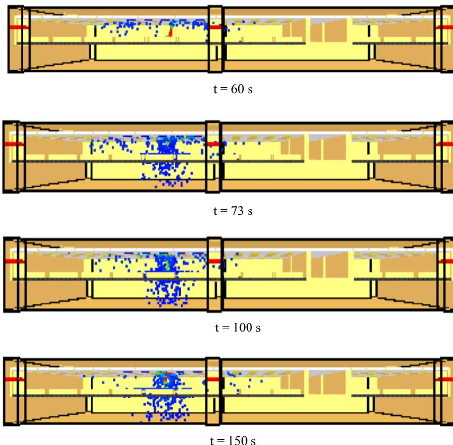
Fig. 10: The smoke particles profiles within temperature (scenario 3)
