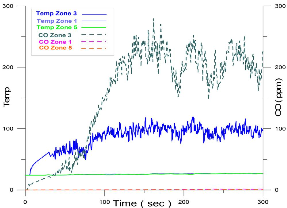
Fig. 11b: The temperature and CO concentration measured variation at the height near ceiling (scenario 4)
