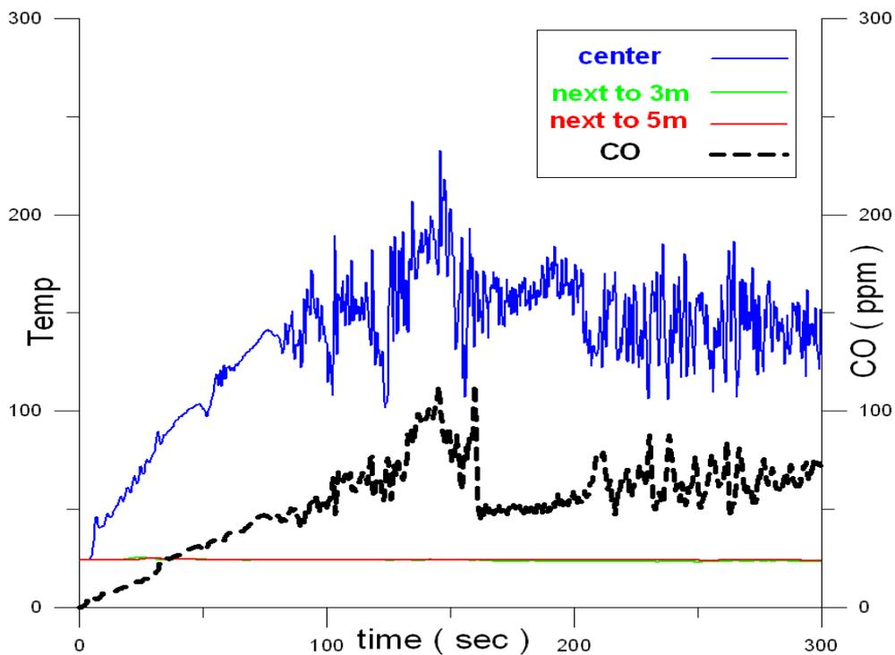
Fig. 7a: The temperature and CO concentration measured variation at 1.8 m (scenario 1)
