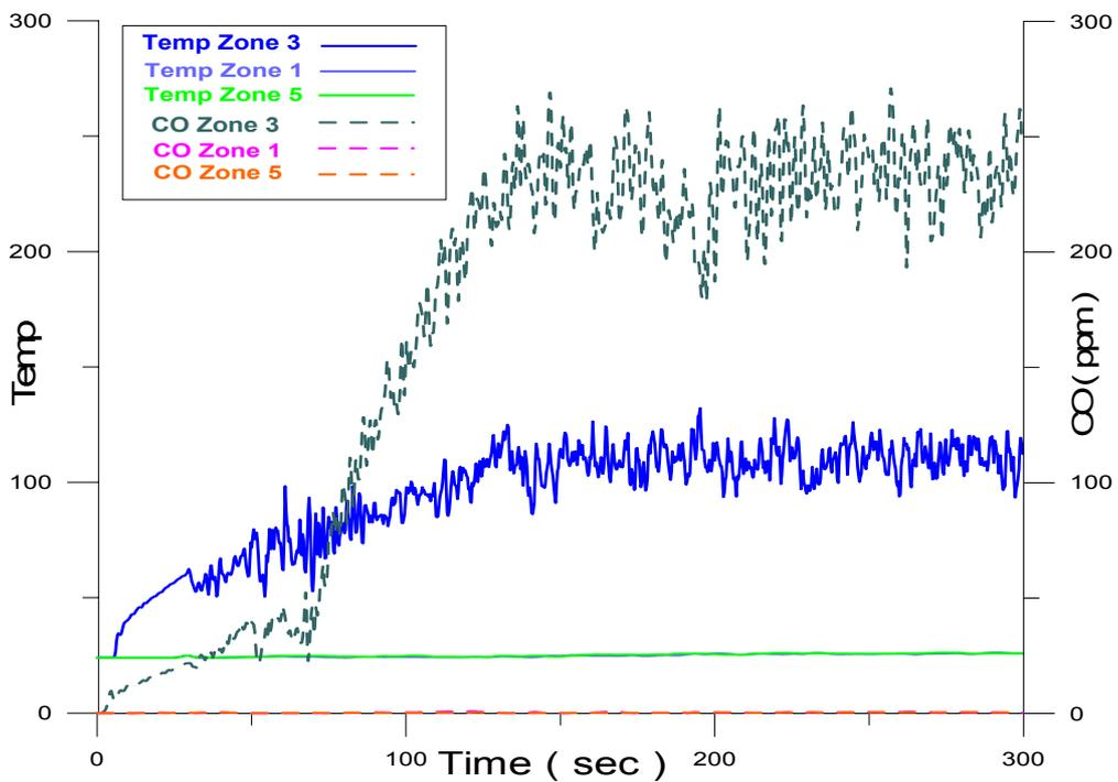
Fig. 9b: The temperature and CO concentration measured variation at the height near ceiling (scenario 3)
