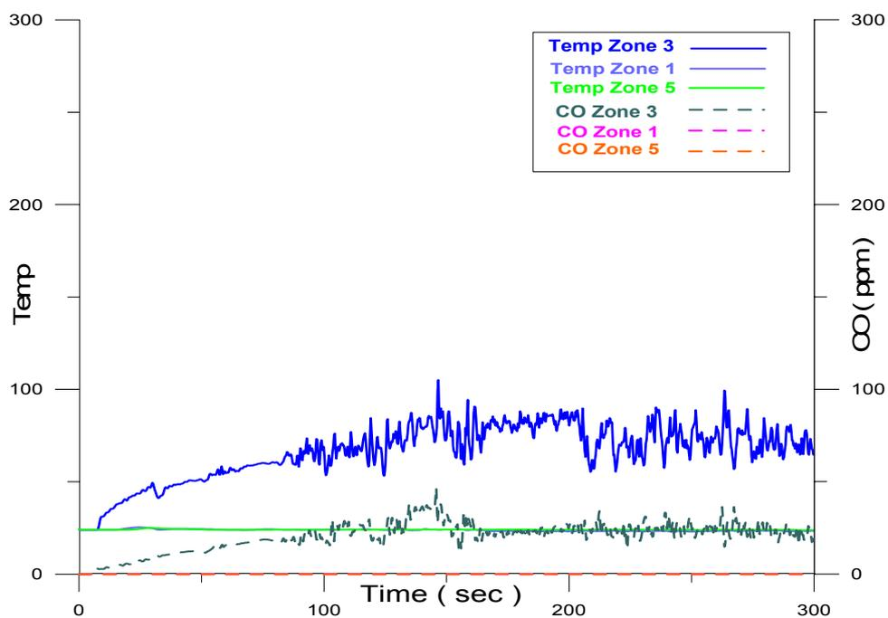
Fig. 7b: The temperature and CO concentration measured variation at the height near ceiling (scenario 1)
