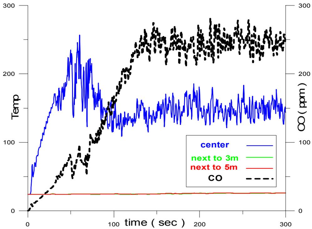
Fig. 9a: The temperature and CO concentration measured variation at 1.8 m (scenario 3)
