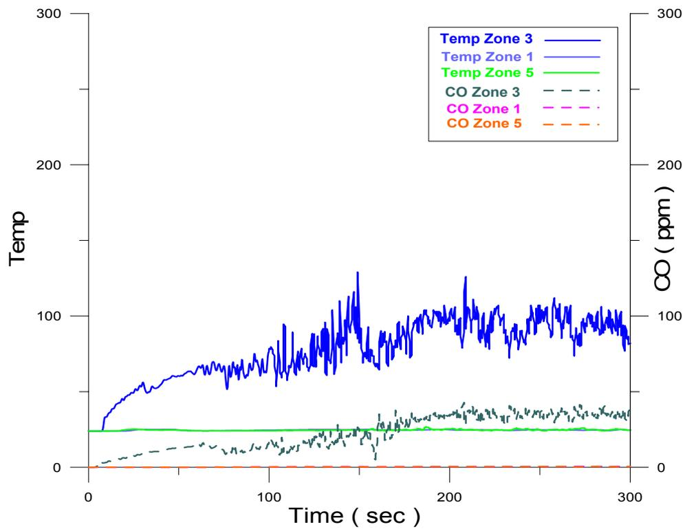
Fig. 8b: The temperature and CO concentration measured variation at the height near ceiling (scenario 2)
