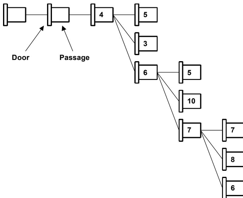
Fig. 2: Example of an evacuation tree
