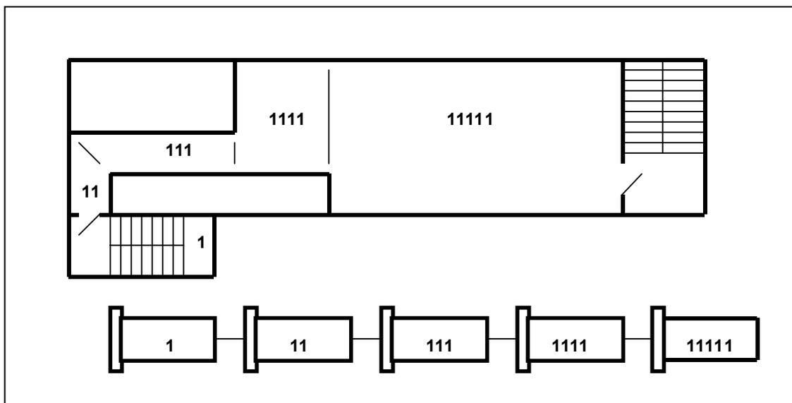
Fig. 8: Modelling of the Disco first floor by a sequence of virtual rooms
