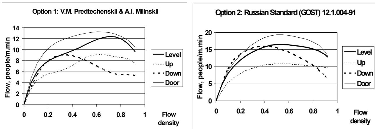
Fig. 1: Dependence of the pedestrian flow on flow density
