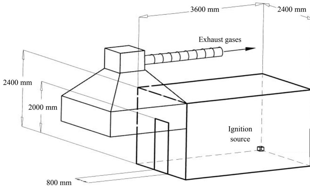
**Fig. 1: Configuration of the ISO 9705 full-scale burning test**
