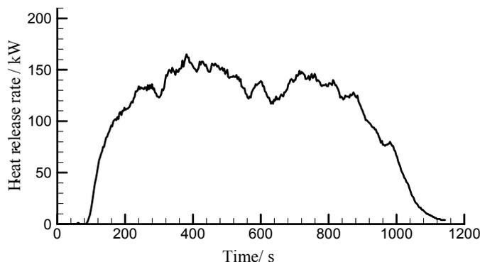
(b) 0.35 m × 0.35 m by 0.25 m high container with 3500 ml gasoline
