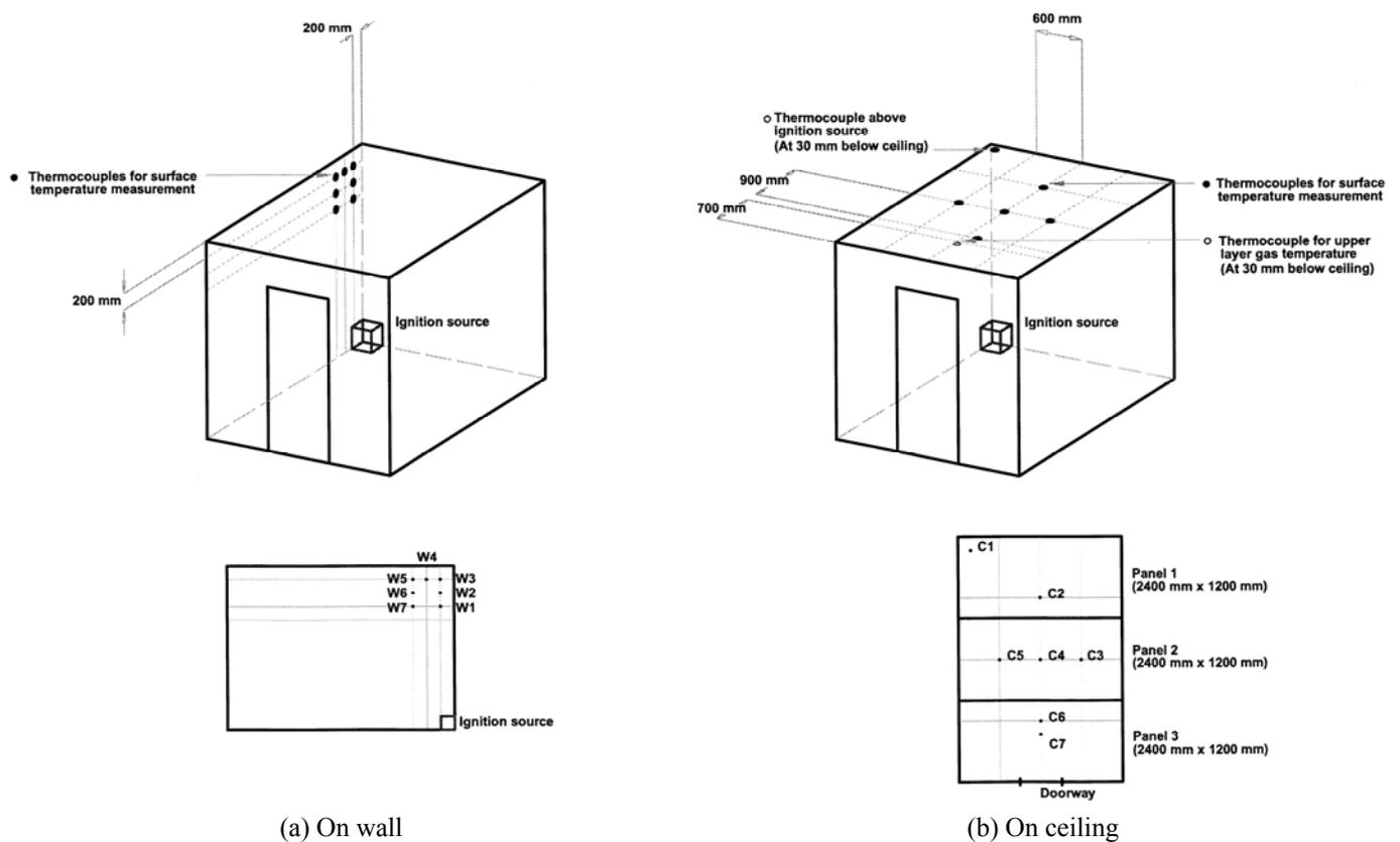
Fig. 4: Locations of thermocouples for measuring wall surface and upper layer gas temperatures
