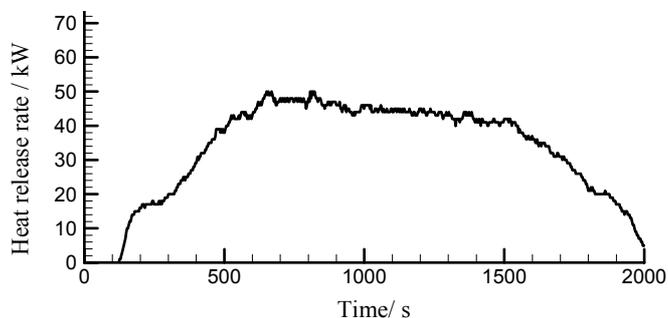
(a) 0.26 m × 0.26 m by 0.26 m high container with 2000 ml gasoline
