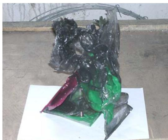
(c) The CD boxes were melted and stuck together
