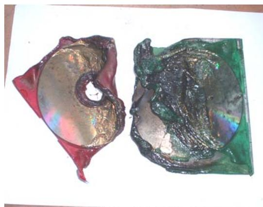
(b) The CD was melted together with the box
