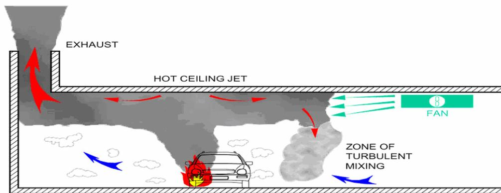
**Fig. 3: Impulse (or Jetfan) smoke ventilation**
