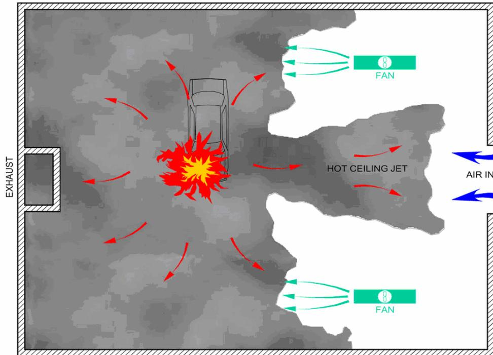
**Fig. 4: Impulse (or Jetfan) smoke ventilation**
