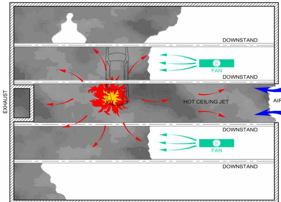
**Fig. 5: Impulse (or Jetfan) smoke ventilation**
