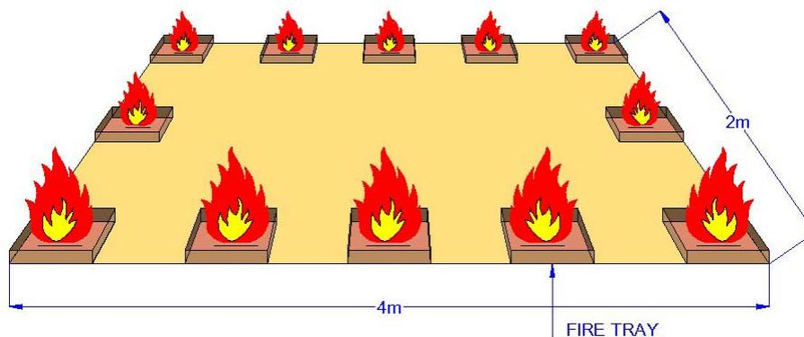
Fig. 8: Fire tray layout for the Car Park example of section 6.4
