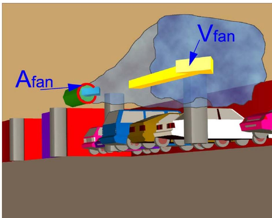
Fig. 7: The exhaust jet from a jetfan mounted close beneath a car park ceiling
