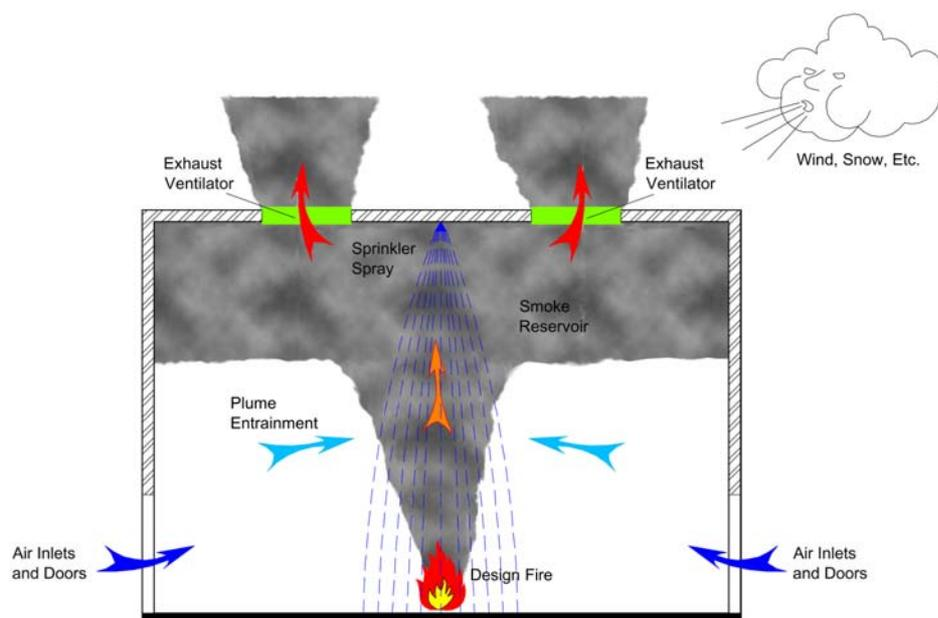
Fig. 1: The principles of smoke and heat exhaust ventilation
