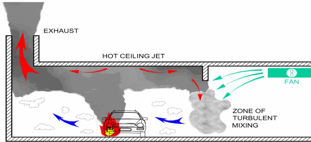
**Fig. 6: Impulse (or Jetfan) smoke ventilation**
