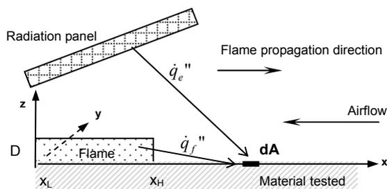
Fig. 3: Basic geometry and coordinate system of the flame spreading model
