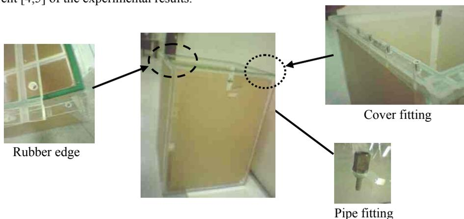
Fig. 1: Details of the acrylic model
