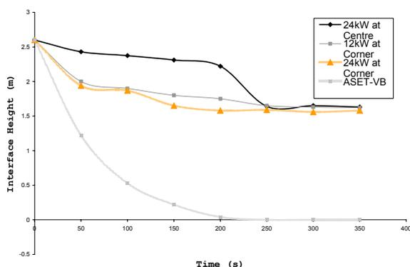
Fig. 11: Comparison of interface height between the 24 kW and 12 kW heater and ASET
