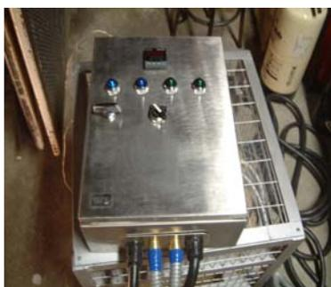
Fig. 4: Thermal controller
