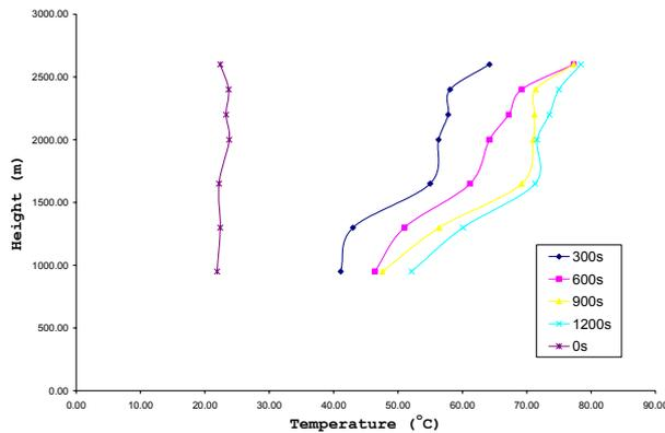
Fig. 9: Temperature profile of the fire chamber
