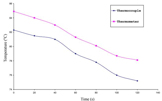
**Fig. 2: Calibration of thermocouple K**
