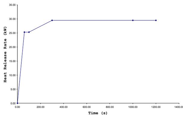
Fig. 10: Heat release rate of the 24 kW heater against time
