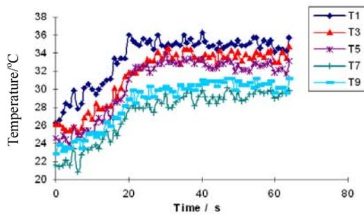
Fig. 6: Vertical temperature profile with no vent
