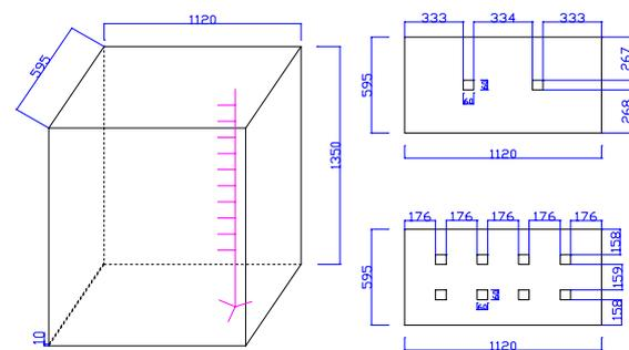
**Fig. 1: Dimensions of scaled model and ceiling plates**
