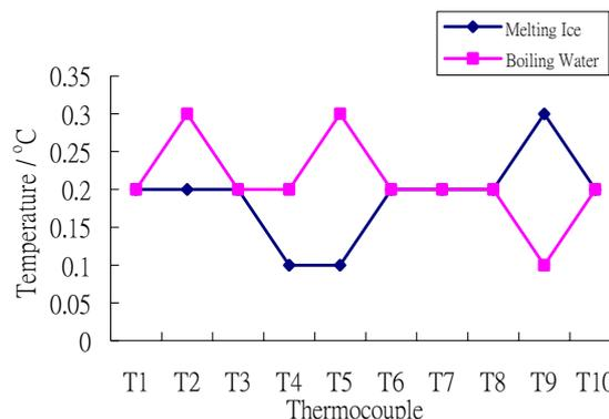
Fig. 4: Errors of thermocouples
