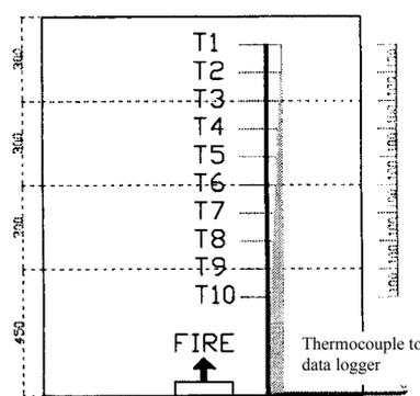
Fig. 5: Measurement of vertical temperature profile and position of taking descending time
