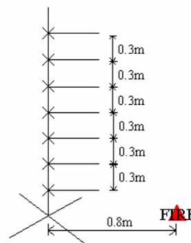
Fig. 1: K-type thermocouple tree
