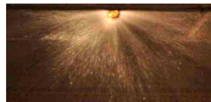
Fig. 4: Water discharge pattern
