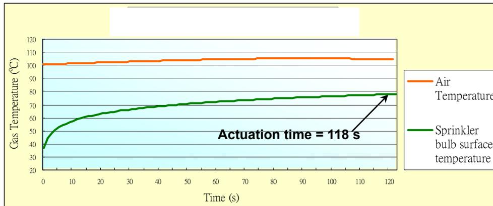
Fig. 10: Typical results of concealed type sprinkler on the temperature-time curve (110 °C, 3 ms<sup>-1</sup>)
