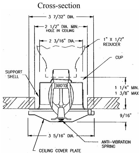
Fig. 3: The concealed sprinkler (captured from Globe Catalogue)
