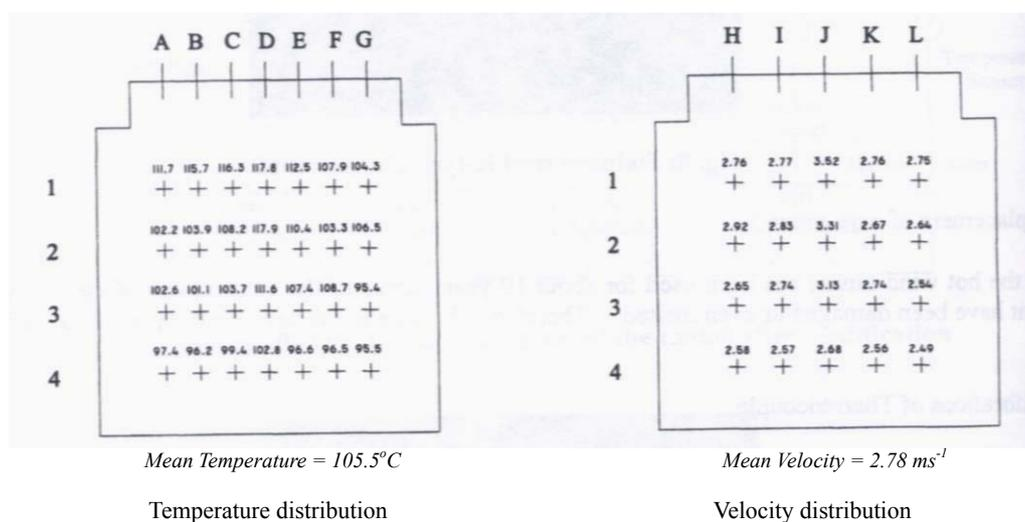
**Fig. 9: Temperature and velocity distribution in the working section of the hot wind tunnel**
