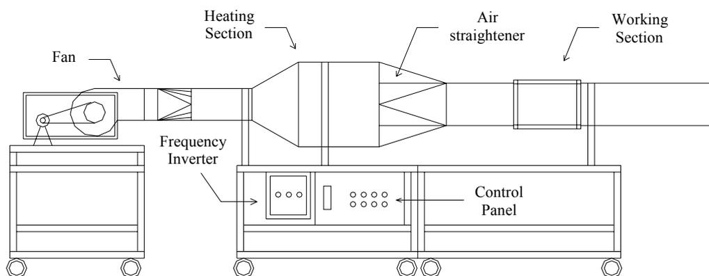
**Fig. 4: The BSE hot wind tunnel**
