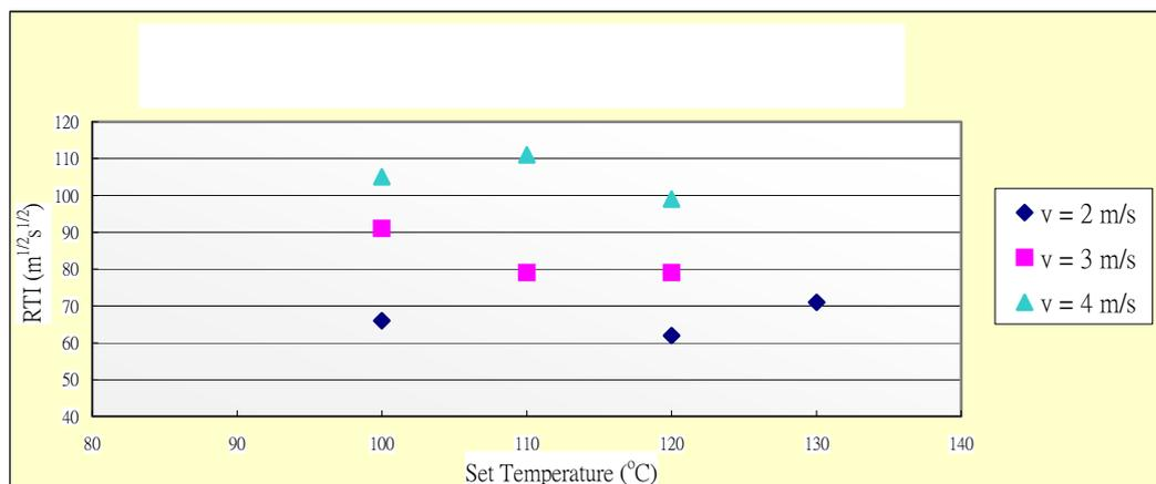
Fig. 11: RTI of pendent type sprinkler head against set temperature
