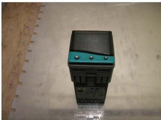
Fig. 6: The PID controller
