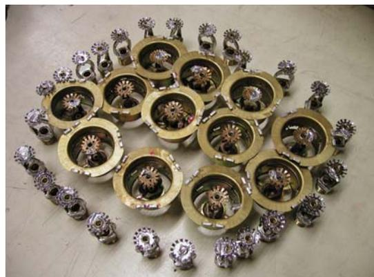
Fig. 2: The tested sprinkler heads
