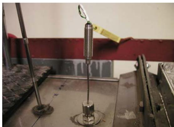
Fig. 8: Stainless steel K-type thermocouple
