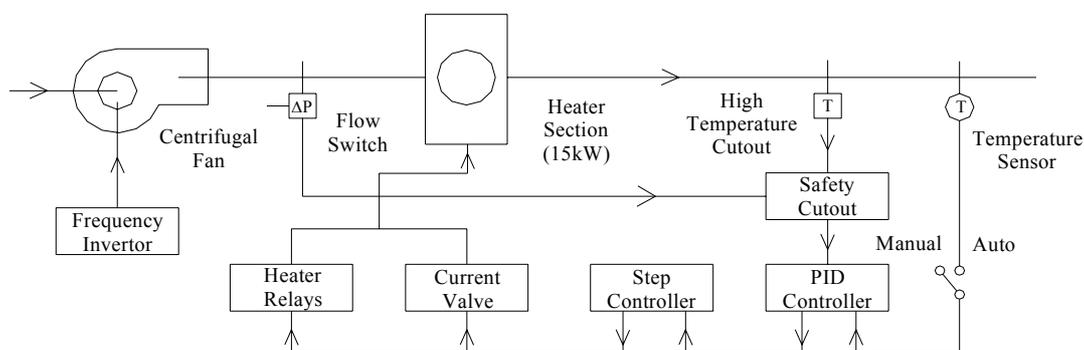
**Fig. 5: The simplified control logic diagram of the tunnel after modification**
