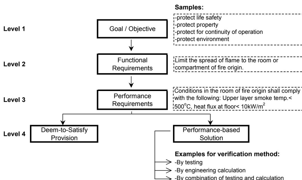
Fig. 1: The general four-level regulatory framework [29]
