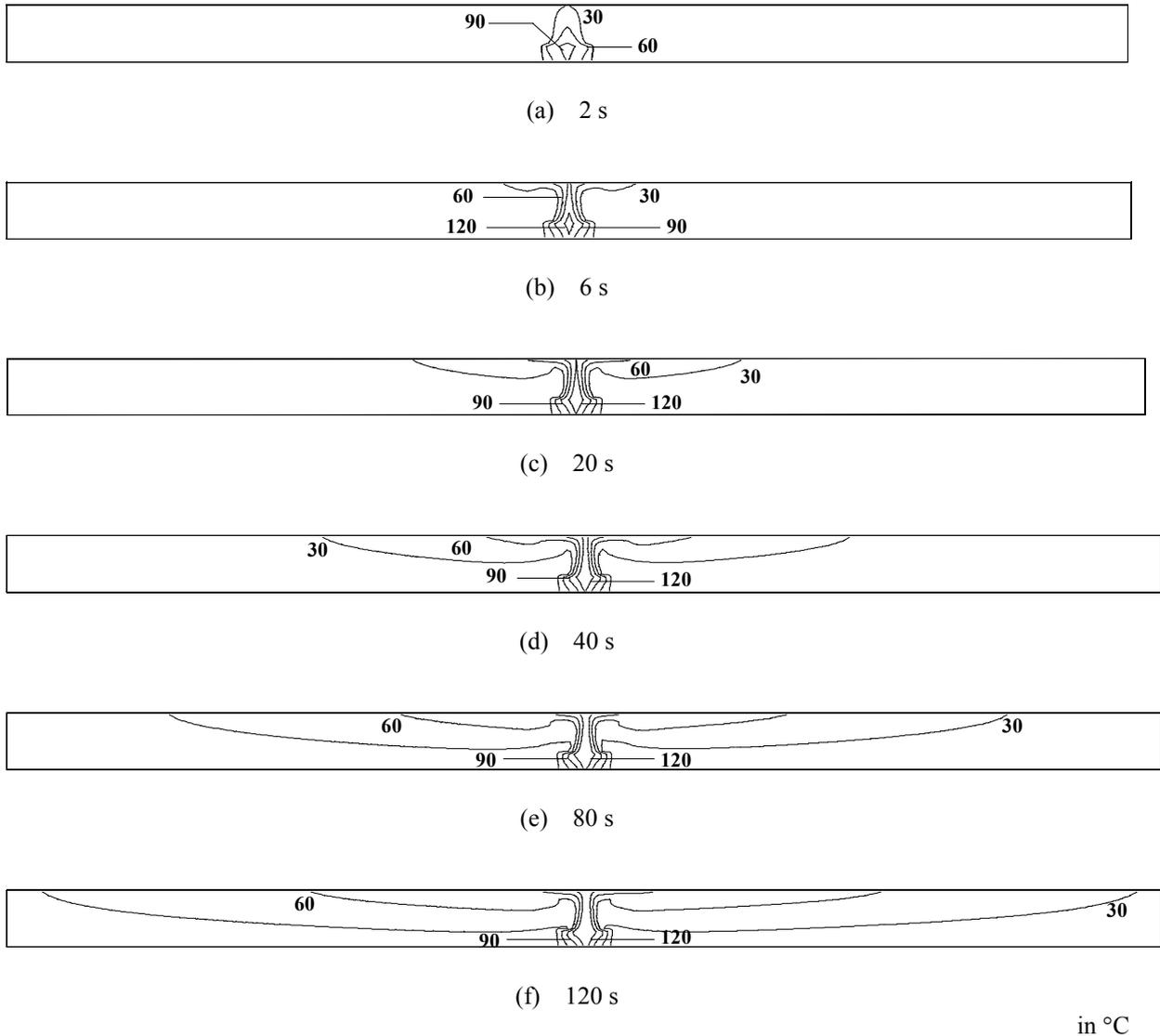
Fig. 2: Temperature contours of the tunnel with a 0.5 MW fire
