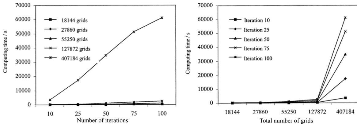
Fig. 6: Computing time of CFD in relation to the number of iterations and grids
