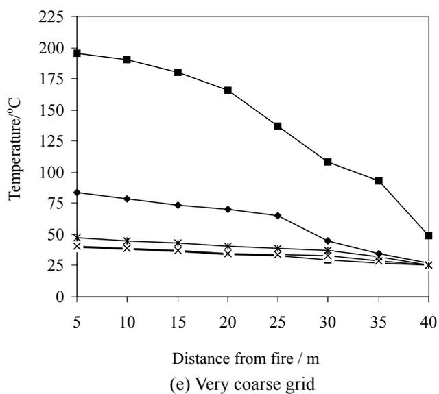
Fig. 5: Grid variation on air temperature in the middle part of the tunnel
