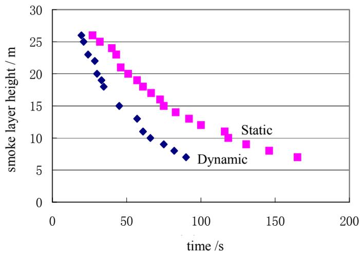
(b) Comparison between static and dynamic smoke exhaust
