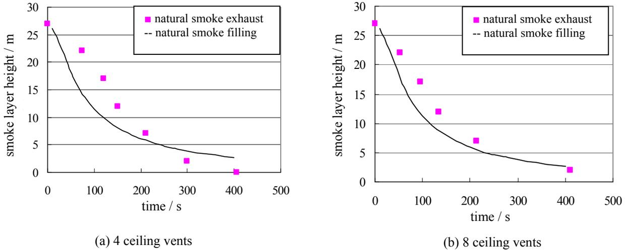
Fig. 3: Natural smoke exhaust for a 1.2 MW pool fire
