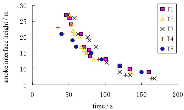
Fig. 7: Smoke layer interface height under different positions and areas of air inlets
