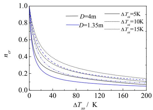
(b) Temperature difference between indoor lower air layer and outdoor ambient air is not zero
