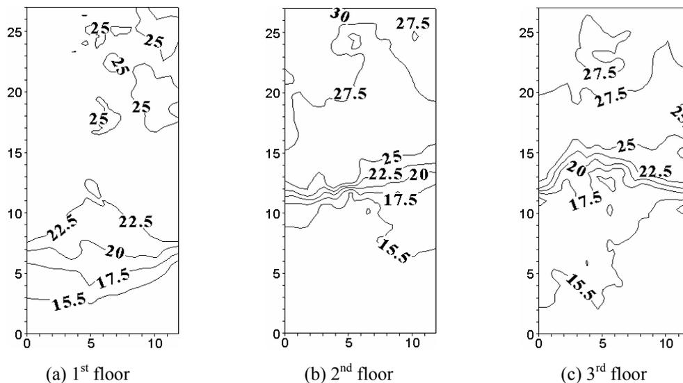
Fig. 6: Temperature distribution predicted by FDS-2 with different positions of air inlets
