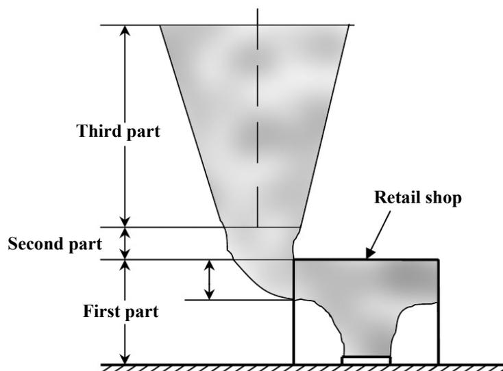
Fig. 10: The three parts of a self-developed plume model
