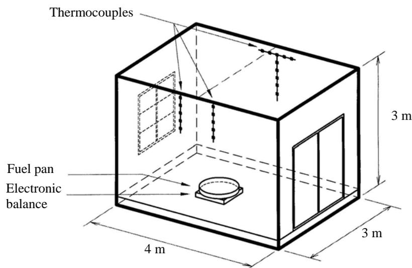
**Fig. 2: Geometry of small chamber inside the Atrium**
