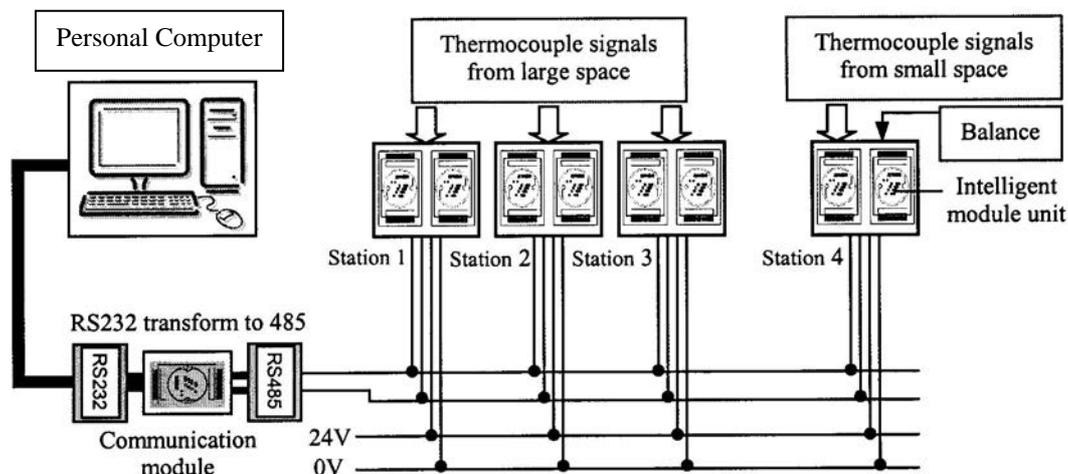
**Fig. 3: Schematic diagram of the data acquisition system**
