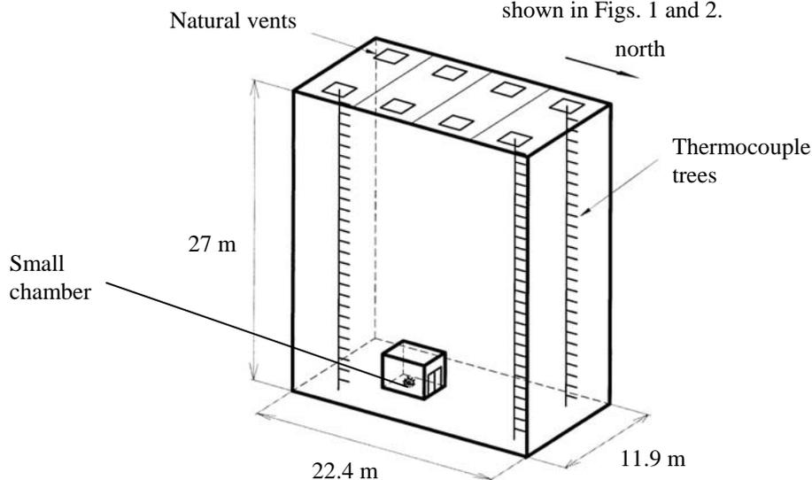
**Fig. 1: Geometry of PolyU/USTC Atrium**
