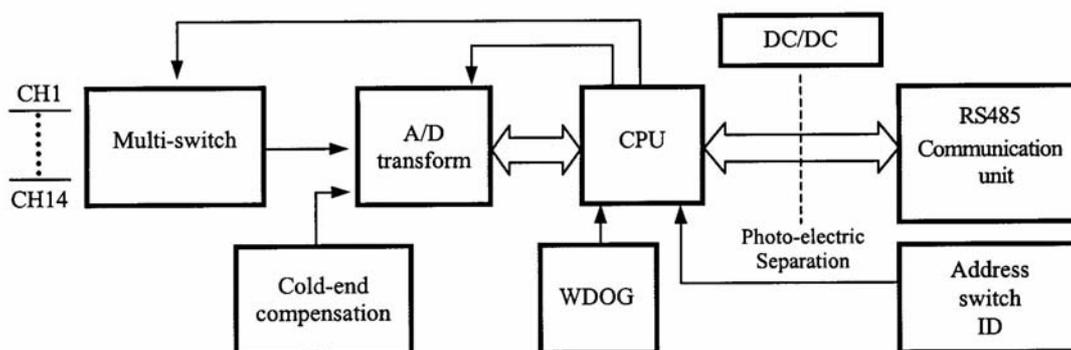
**Fig. 4: Schematic diagram of the intelligent module RM410**
