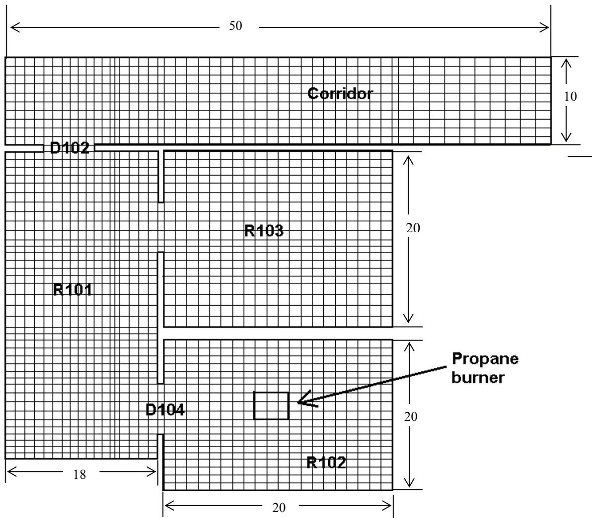
Fig. 2: Mesh layout for the simulations
