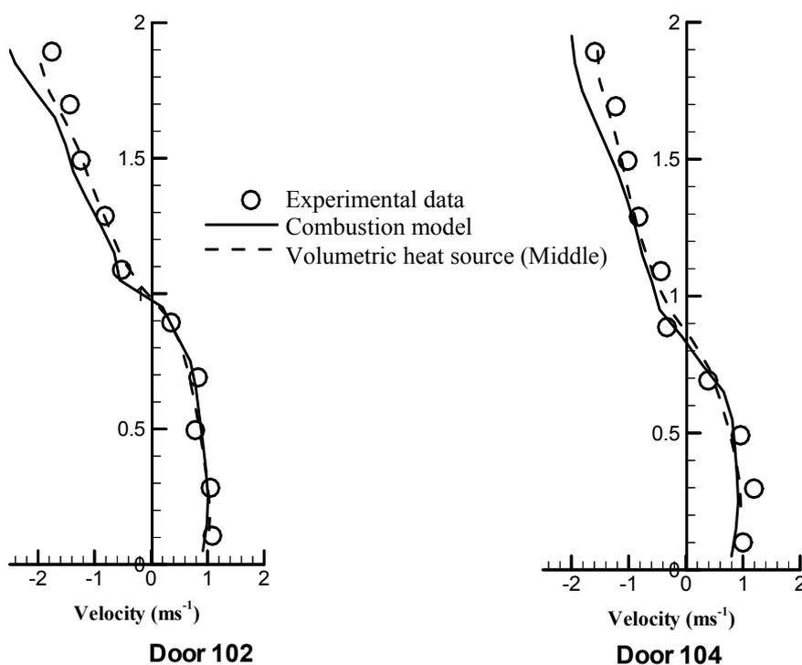
Fig. 6: Comparison of the measured and predicted velocities at Doors 102 and 104
