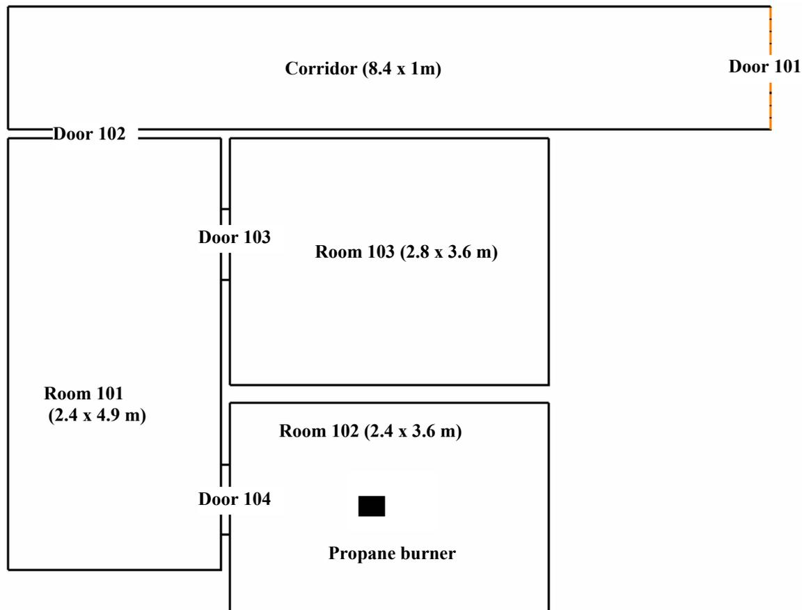
Fig. 1: Layout of the experimental facility conducted by Luo & Beck (1994)
