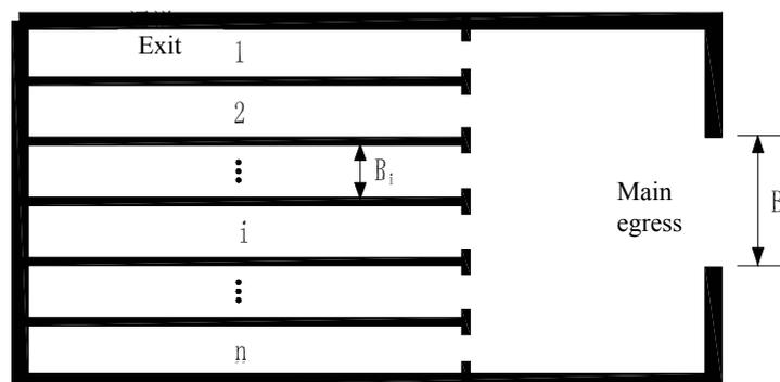
Fig. 1: Simplified model of a highrise building plan
