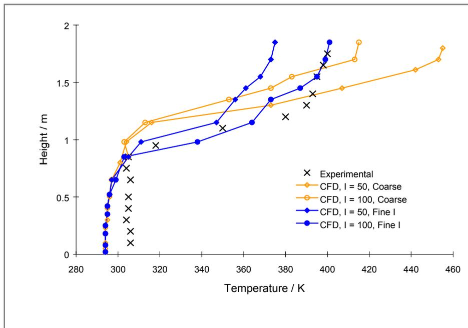
(a) With cell refinement at fire source
