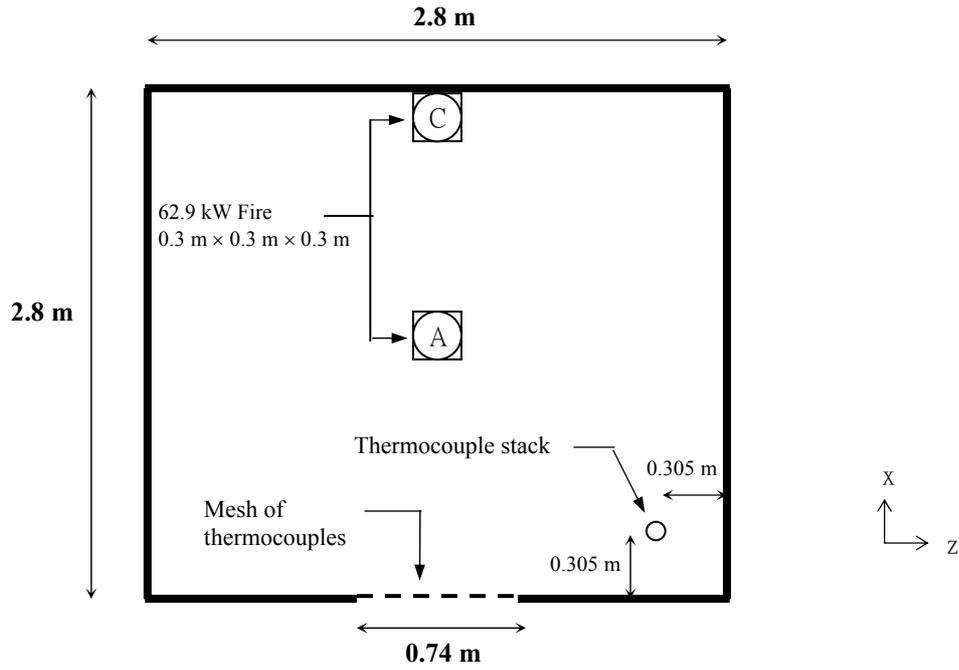
Fig. 1: Configuration of experiment by Steckler et al.
