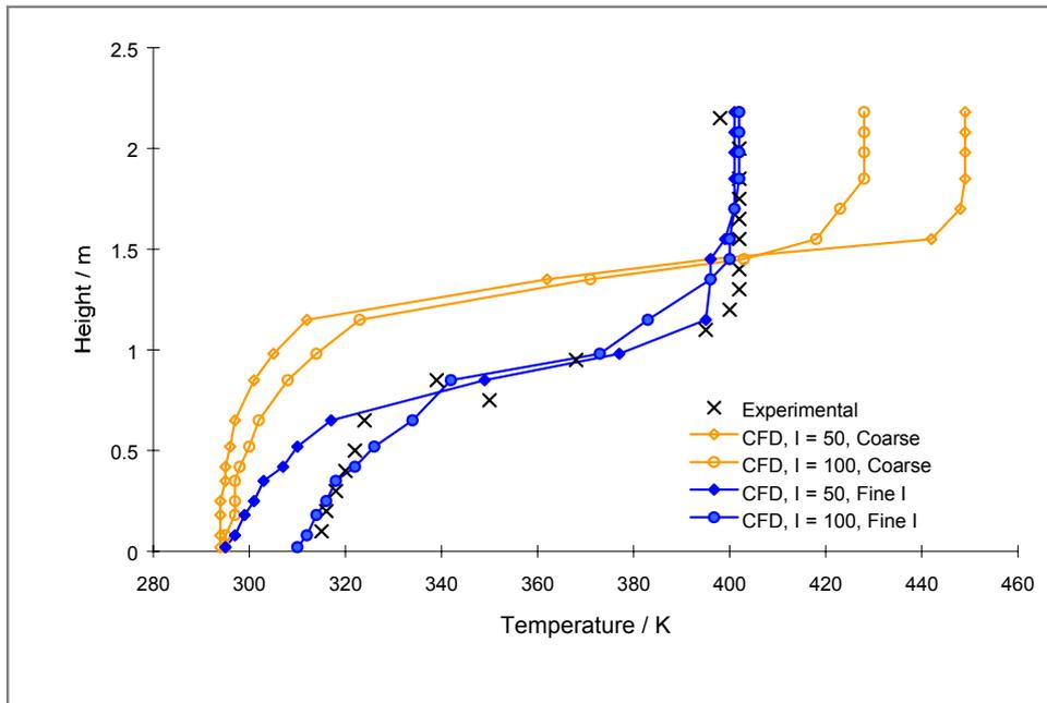
(a) With cell refinement at fire source
