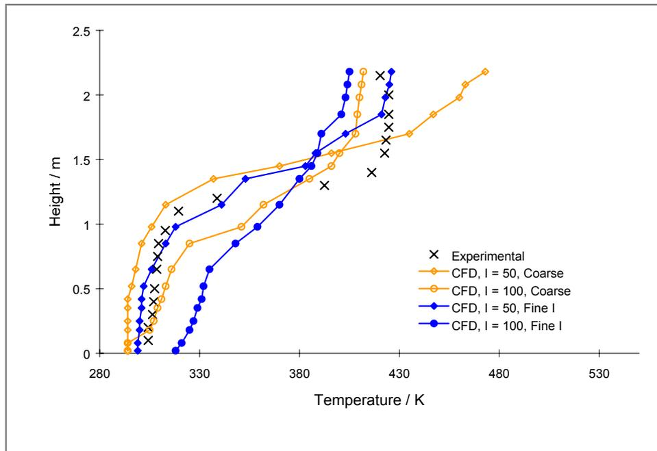
(a) With cell refinement at fire source
