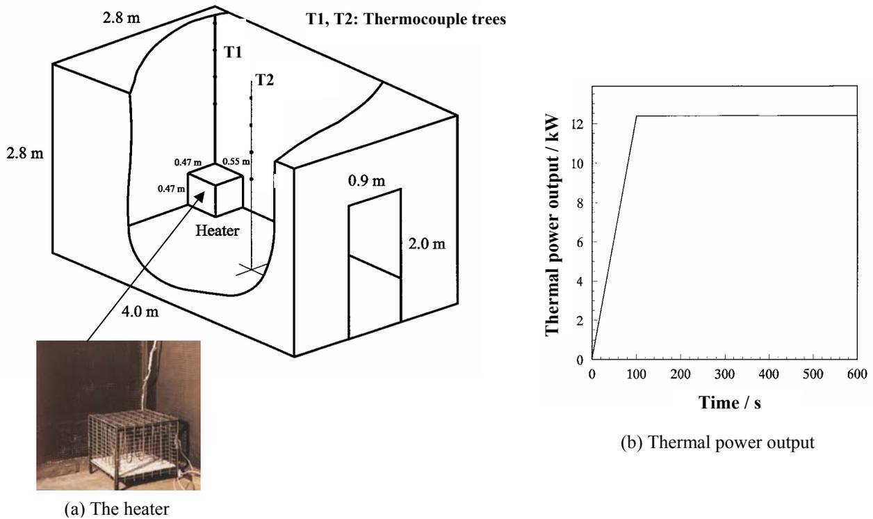
Fig. 1: Geometry of fire chamber
