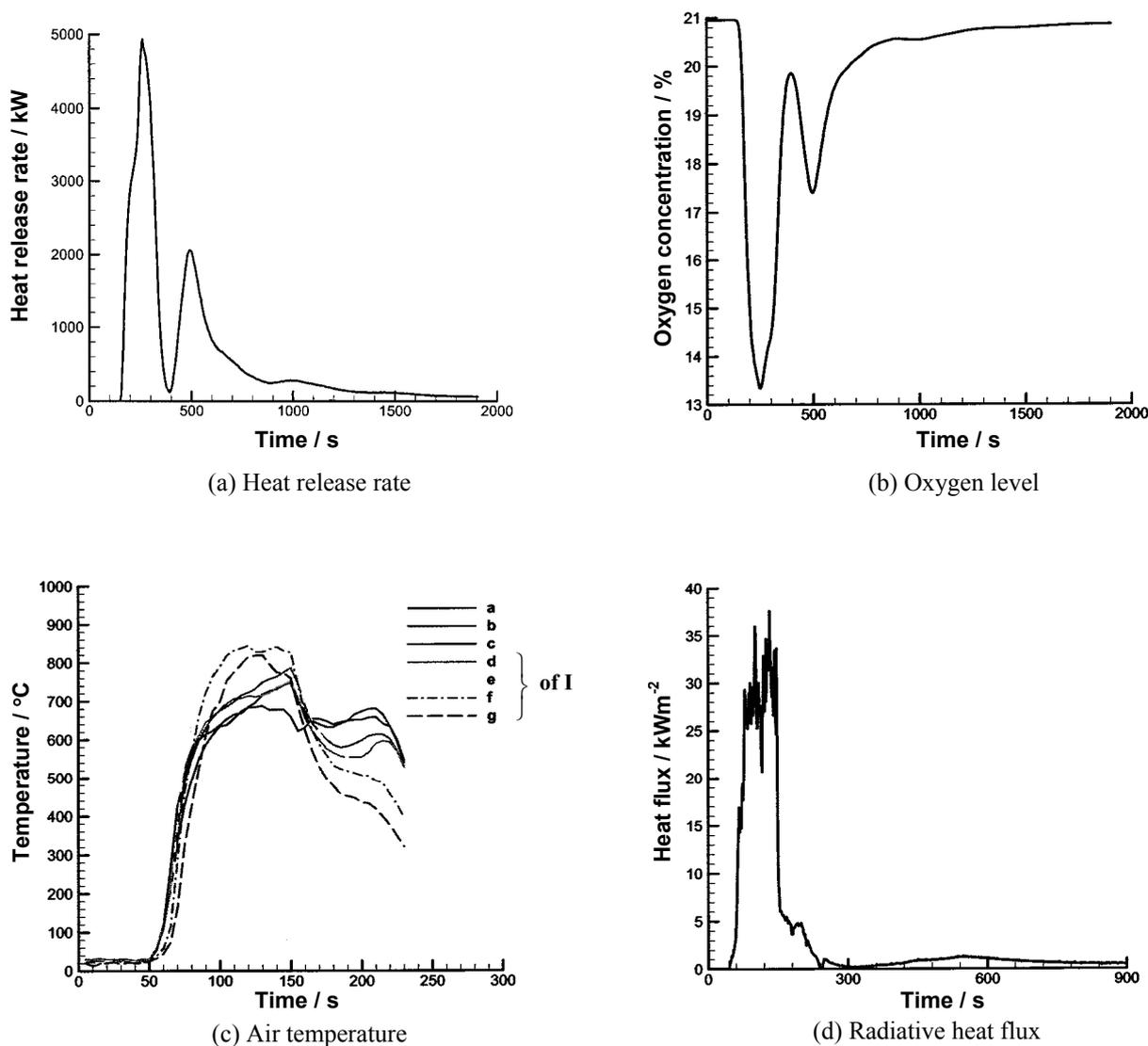
Fig. 5: Results for test 3 with water mist discharged
