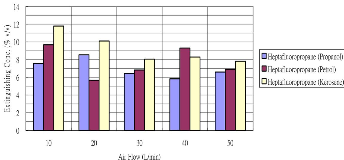
Fig. 1: Extinguishing concentration of heptafluoropropane against different fuels with small cup and large chimney (agent flow rate = 15 L/min)
