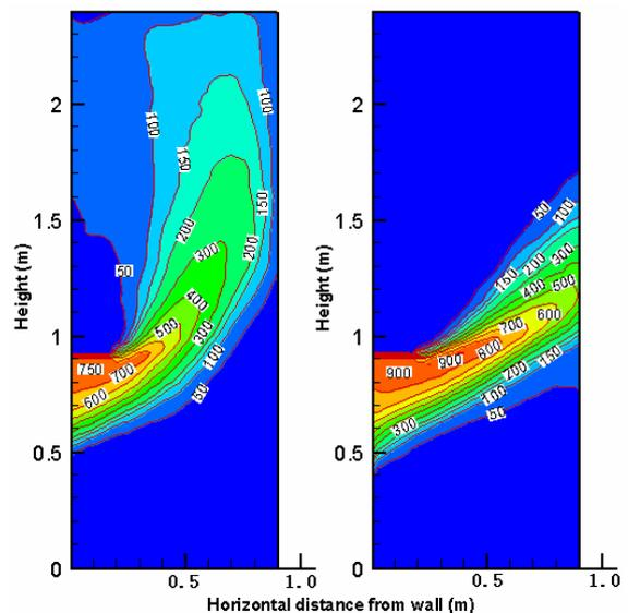
Fig. 5: Temperature distributions with wind effects
