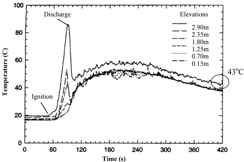
Fig. 2: Room temperature for pool fire with door open
