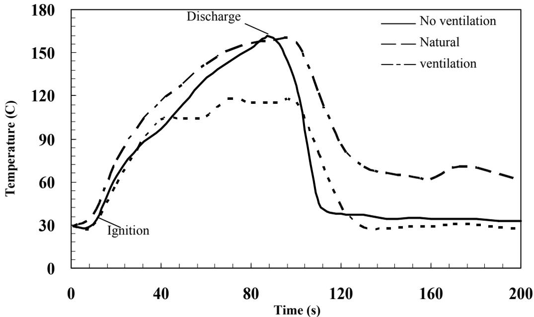
Fig. 3: Room temperature for pool fire with different ventilation conditions
