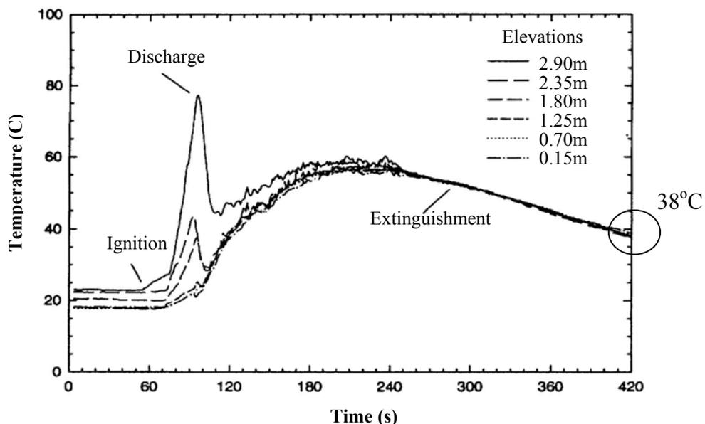
Fig. 1: Room temperature for pool fire with door closed
