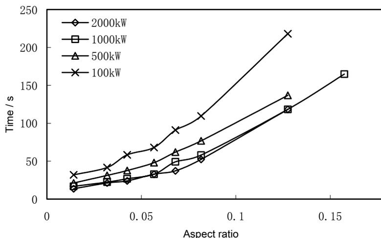
**Fig. 5: Relation between the time when flooding flow occurred and  $\gamma_f$  of the atrium under different HRR of fire**
