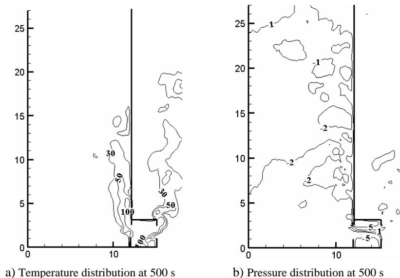
**Fig. 4: Part of the simulation results (atrium of  $12\text{ m} \times 12\text{ m} \times 27\text{ m}$  with HRR of  $1000\text{ kW}$ )**
