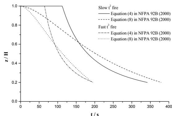
**Fig. 2: Comparison of the smoke filling process predicted by different method for t-squared fire occurring on the atrium floor**
