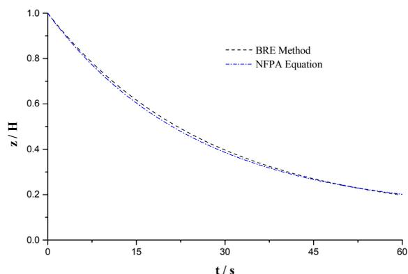
**Fig. 3: Comparison of the smoke filling process predicted by different spill plume equations for steady fire occurring in the adjacent room**
