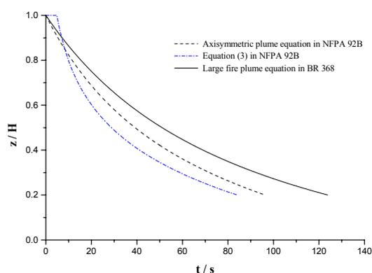
**Fig. 1: Comparison of the smoke filling process predicted by different methods for steady fire occurring on the atrium floor**
