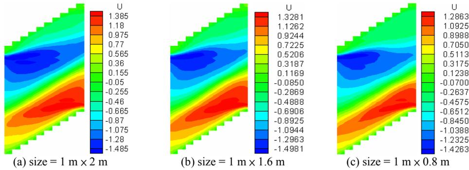
Fig. 6: Nephogram of velocity distribution with various door sizes
