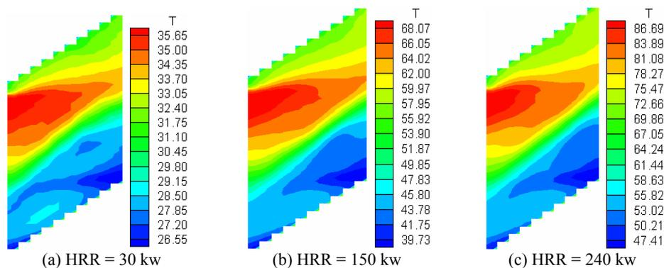
Fig. 3: Nephogram of temperature distribution with various HRR
