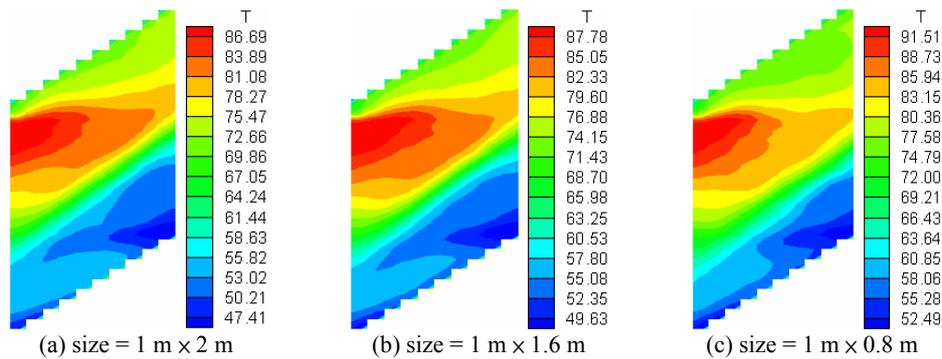
Fig. 7: Nephogram of temperature distribution with various door sizes
