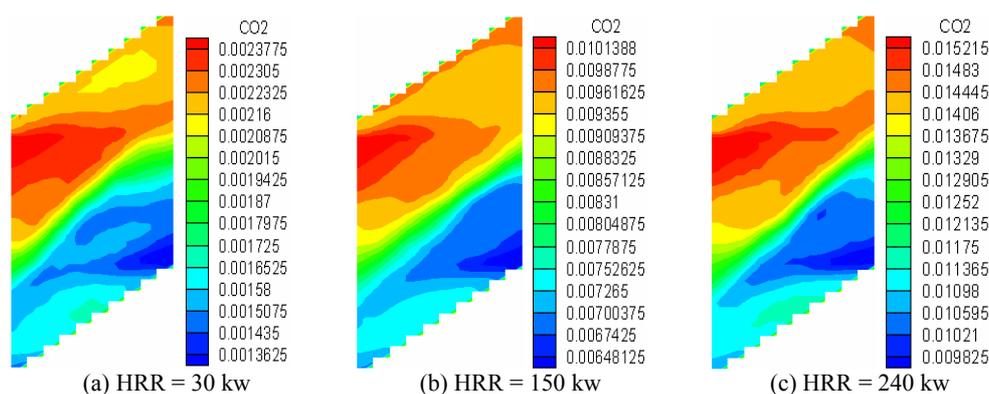
Fig. 5: Nephogram of CO<sub>2</sub> concentration distribution with various HRR
