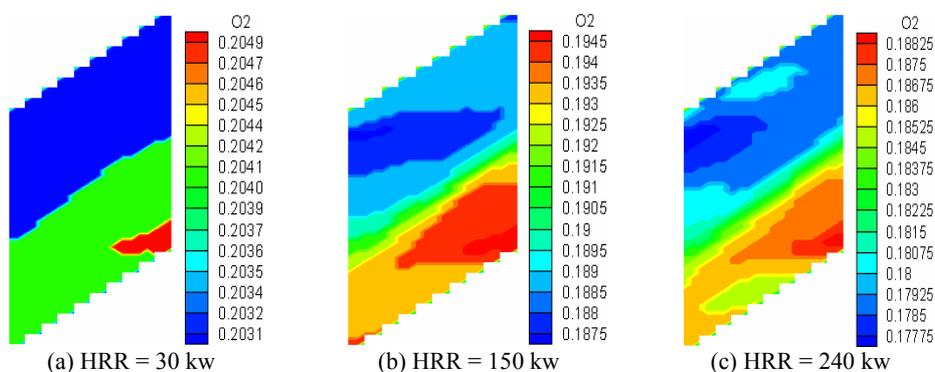
Fig. 4: Nephogram of O<sub>2</sub> concentration distribution with various HRR
