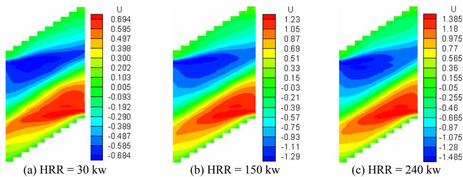
Fig. 2: Nephogram of velocity distribution with various HRR
