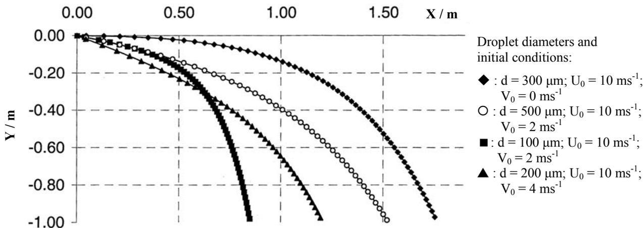
Fig. 4: Selected droplet trajectories in a 300 K smoke layer (layer depth is 1 m)
