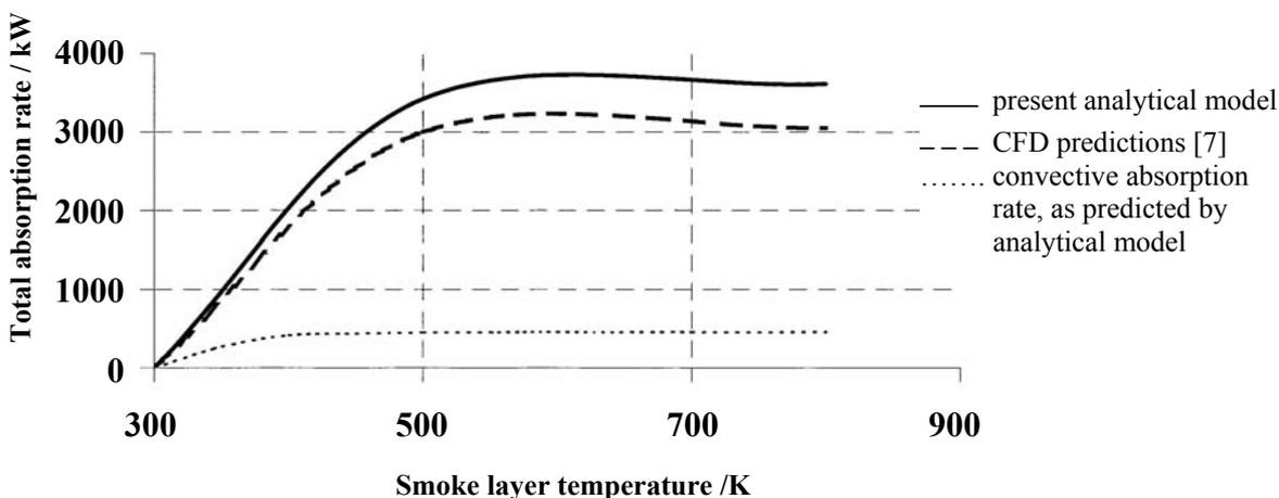
Fig. 6: Heat absorption rate predictions for the AM24 nozzle (layer depth is 1 m; water discharge rate is equal to  $\dot{\psi} = 80 \text{ liters/min}$ )
