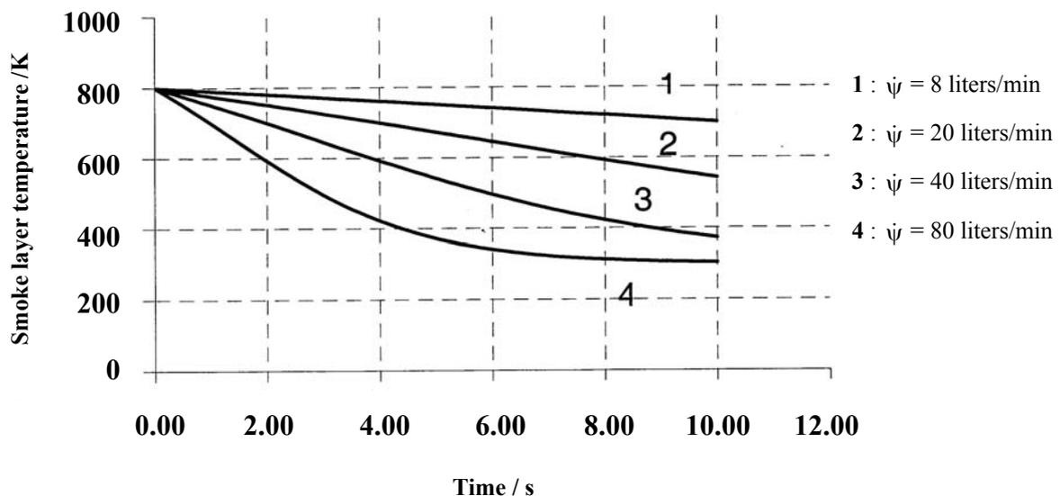
Fig. 7: Smoke layer temperature histories for different water discharge rates (droplet size distribution corresponds to the AM24 nozzle; layer depth is 1 m)
