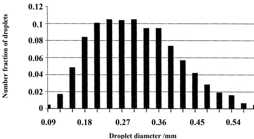
Fig. 5: Droplet size distribution for the AM24 nozzle [8]
