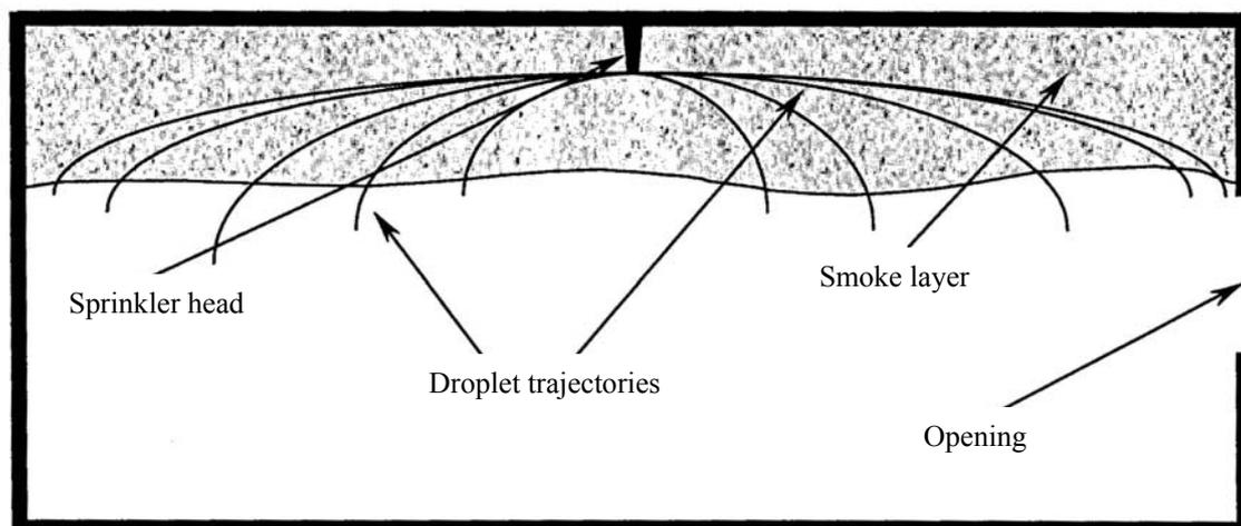
Fig. 1: Schematic view of smoke layer and droplet trajectories in a compartment
