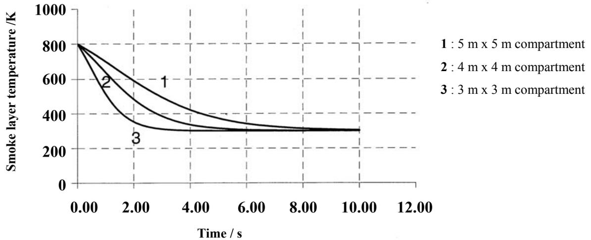
Fig. 8: Effect of the compartment floor area on the smoke temperature drop rate (droplet size distribution corresponds to the AM24 nozzle; layer depth is 1 m; water discharge rate is equal to  $\dot{\psi} = 80$  liters/min)
