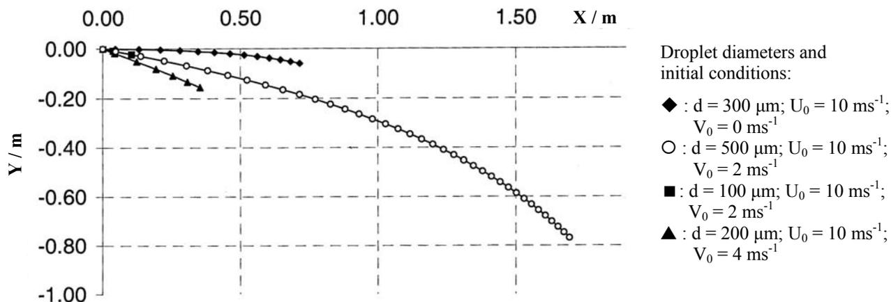
Fig. 2: Selected droplet trajectories in a 800 K smoke layer (layer depth is 1 m)
