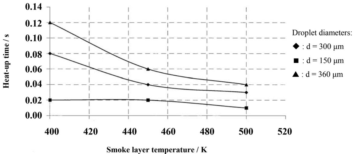
Fig. 9: Heat-up time for various droplets
