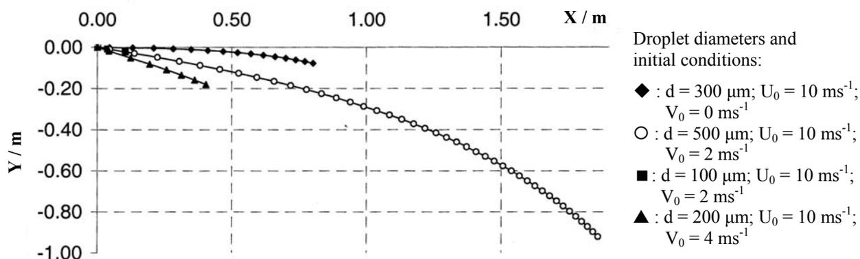
Fig. 3: Selected droplet trajectories in a 500 K smoke layer (layer depth is 1 m)
