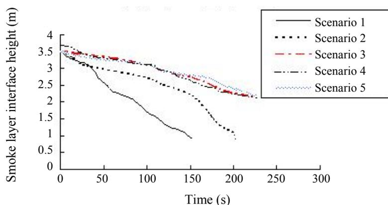
Fig. 3: Variations of smoke layer interface height under different scenarios
