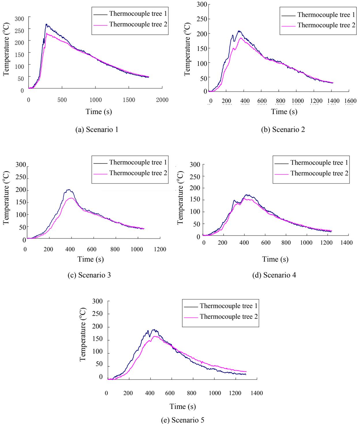
Fig. 5: Horizontal temperature distribution
