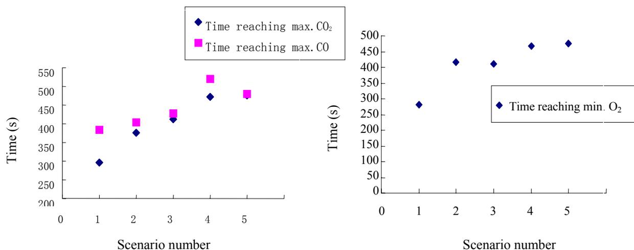
**Fig. 8: Time to reach the maximum and minimum concentration of gases under different scenarios**
