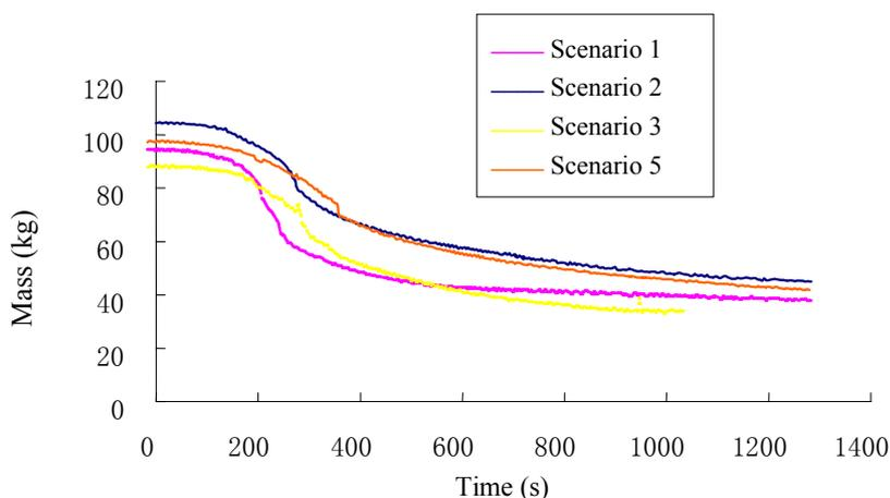
Fig. 2: Rate of mass loss of fire source under different scenarios
