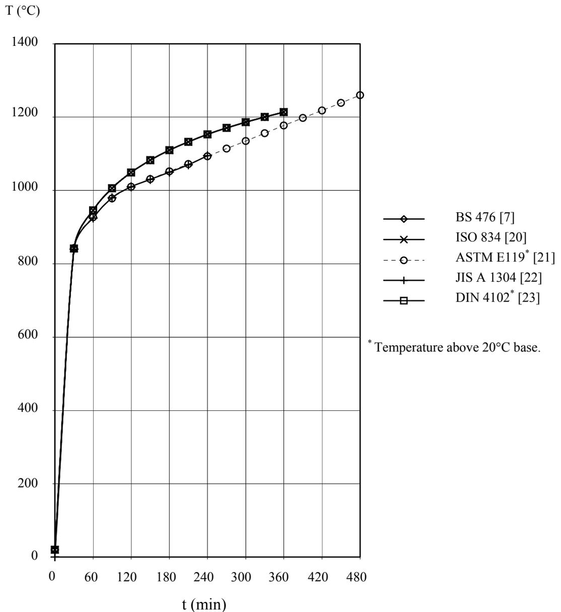
Fig. 3: Comparison of different standard temperature/time curves
