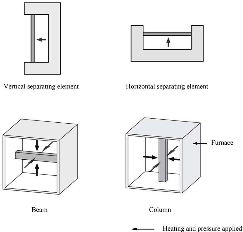
Fig. 2: Heating and pressure applied on test specimen in BS 476
