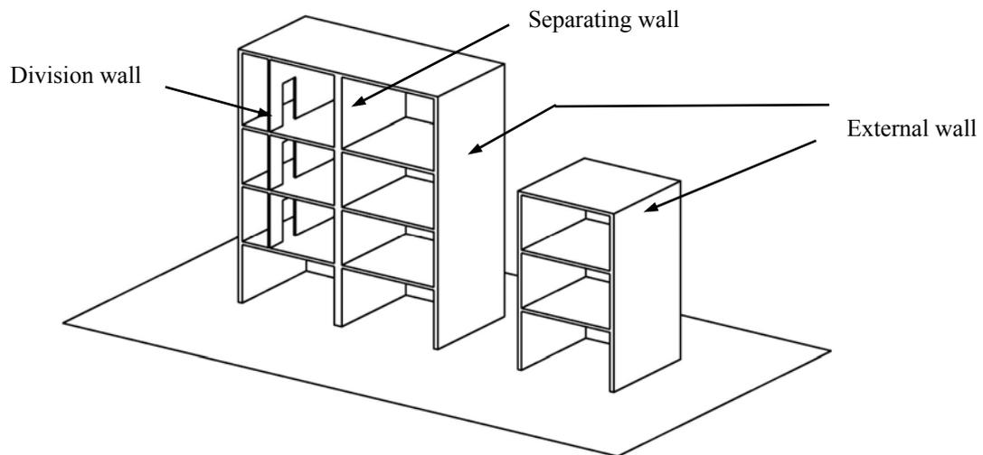
**Fig. 1: Separating wall, division wall and external wall**
