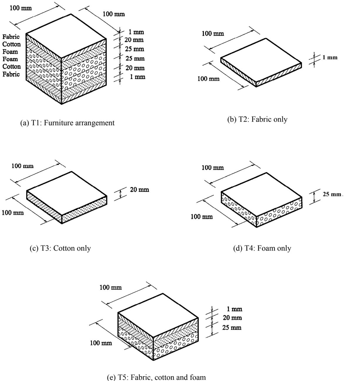
Fig. 1: Geometry of the testing samples
