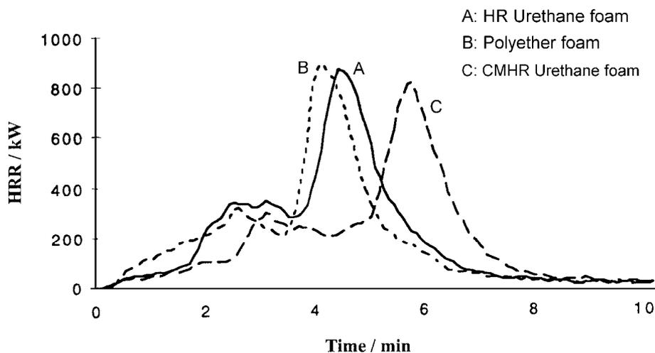
Fig. 1: Heat release rate of different foams (Sundström 1995)
