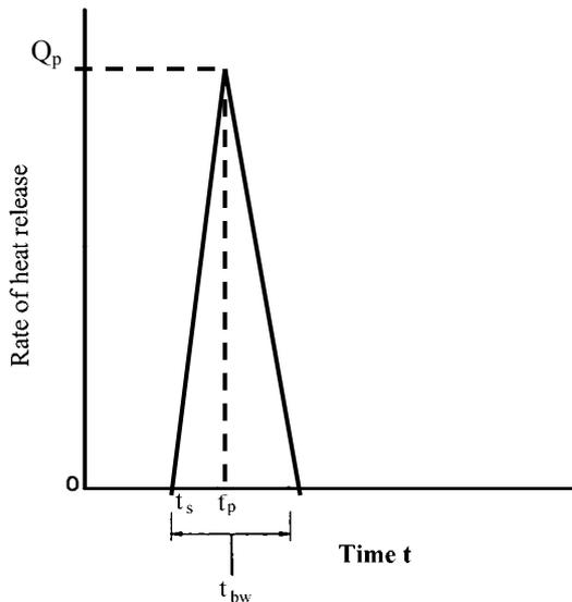
**Fig. 3: Heat release curve for upholstered furniture**
