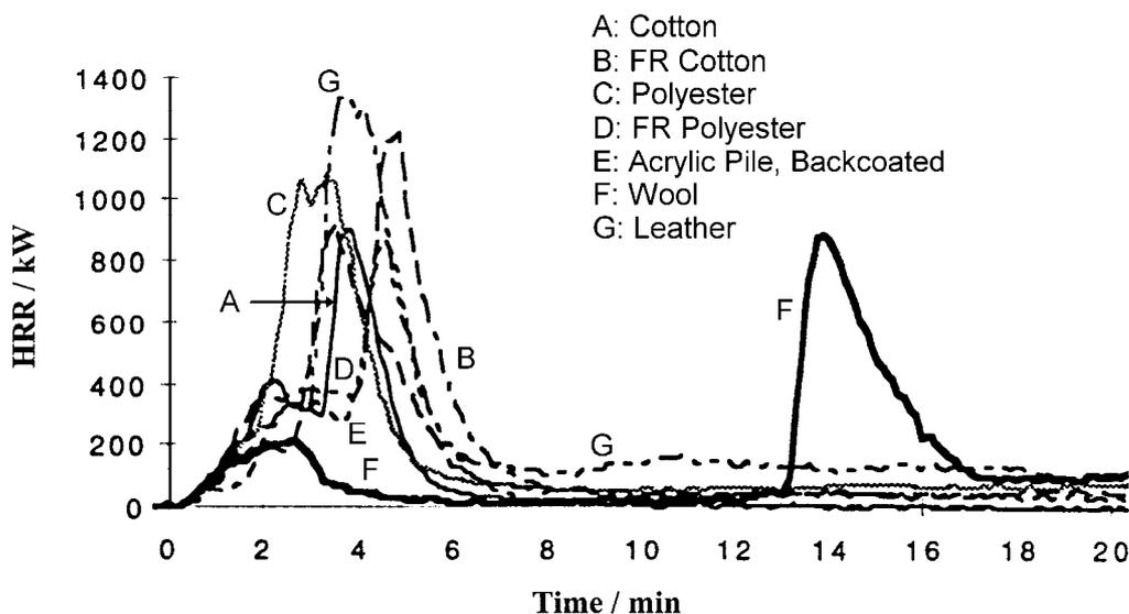
Fig. 2: Heat release rate of different fabrics over high resilient urethane foam (Sundström 1995)
