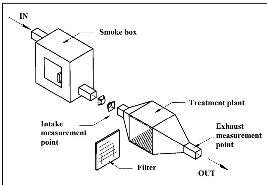
Fig. 2: The basic experimental setup
