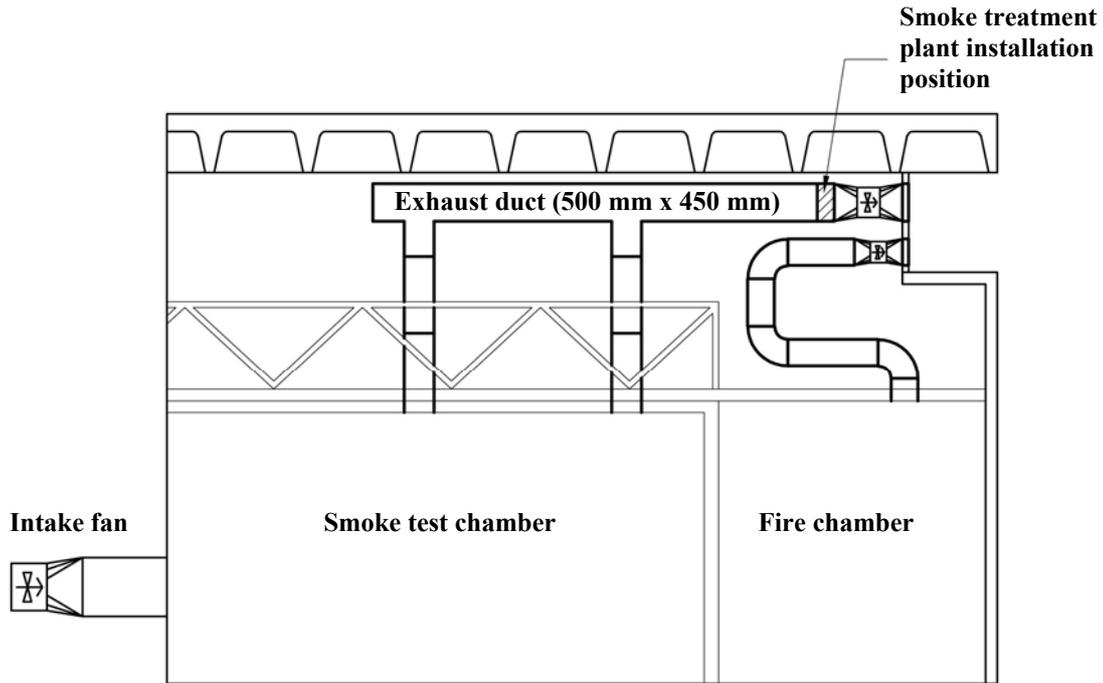
Fig. 4: Section view of the ventilation system at the fire engineering laboratory
