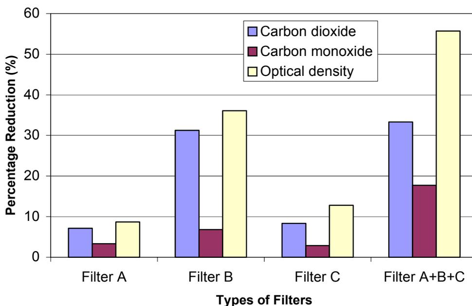
Fig. 3: Cleaning efficiency of filters for smoke treatment plant in percentage reduction
