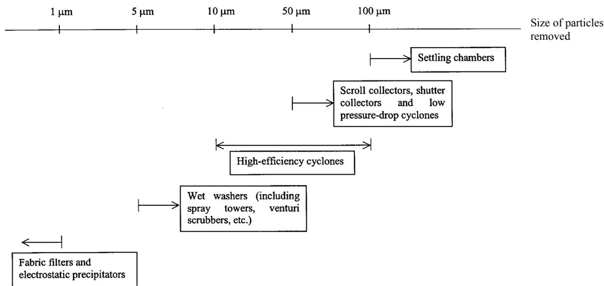
Fig. 1: Pictorial view of dust particulates removal equipment [7]
