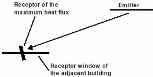
Fig. 1: Receptor and emitter located at an acute angle to each other
