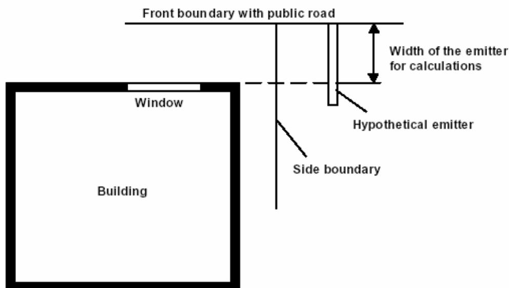
**Fig. 8: Calculations of the heat flux from a hypothetical emitter onto a window facing public road**
