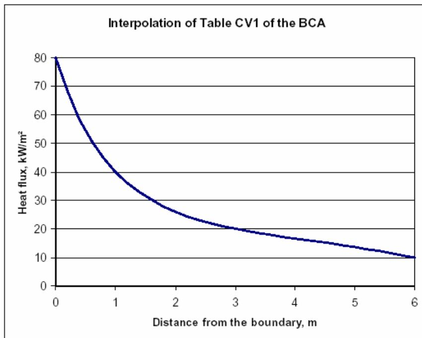
Fig. 7: Interpolation of Table CV1 of the BCA
