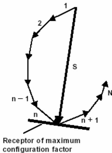
Fig. 3: Heat radiation from several emitters onto a receptor of the maximum configuration factor
