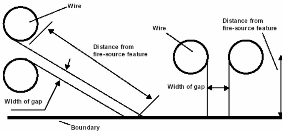
Fig. 6: Comparison of mesh perpendicular to the boundary and facing the boundary
