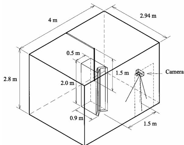
Fig. 1: Equipment setup for droplet velocity measurement
