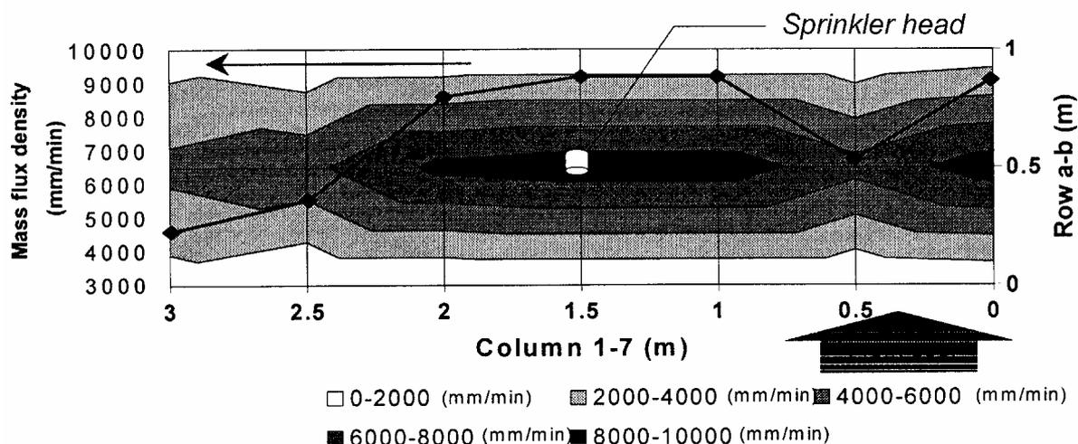
Fig. 4: Mass flux distribution for test C3
