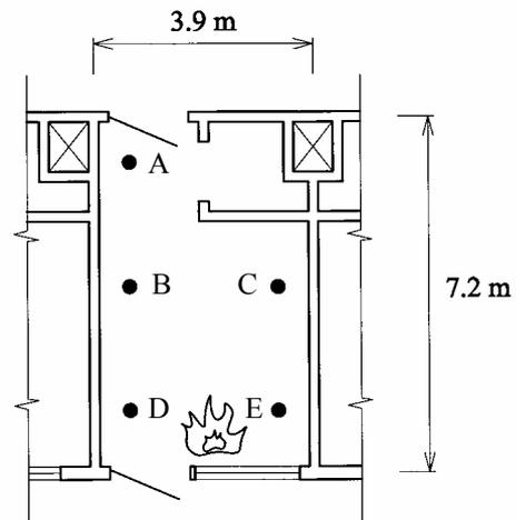
Fig. 5: Plan on the measuring points in the fire room
