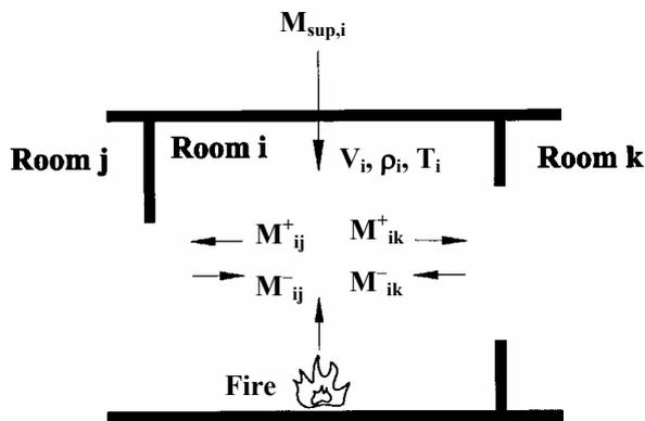
Fig. 1: Mass balancing
