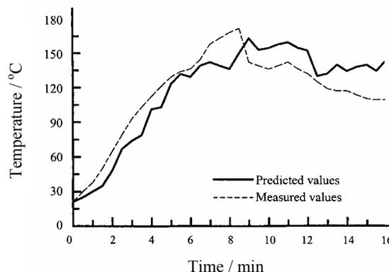
Fig. 7: Fire temperature in the fire room
