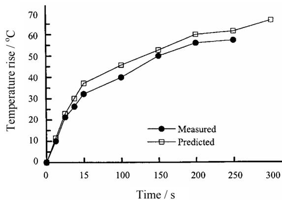
Fig. 9: Average temperature in the fire room for the NIST experiment
