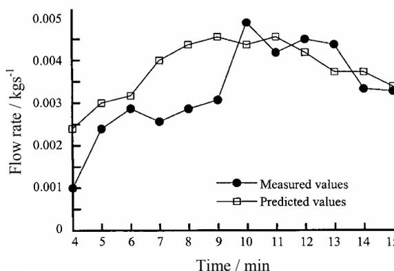
Fig. 8: Mass flow rate
