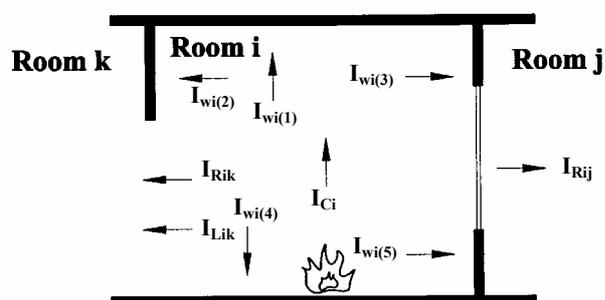
Fig. 2: Heat balancing
