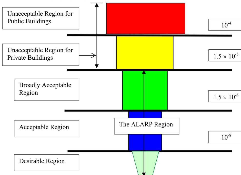
Fig. 1: Fire risk criteria in accordance with DD240 and the ALARP principle
