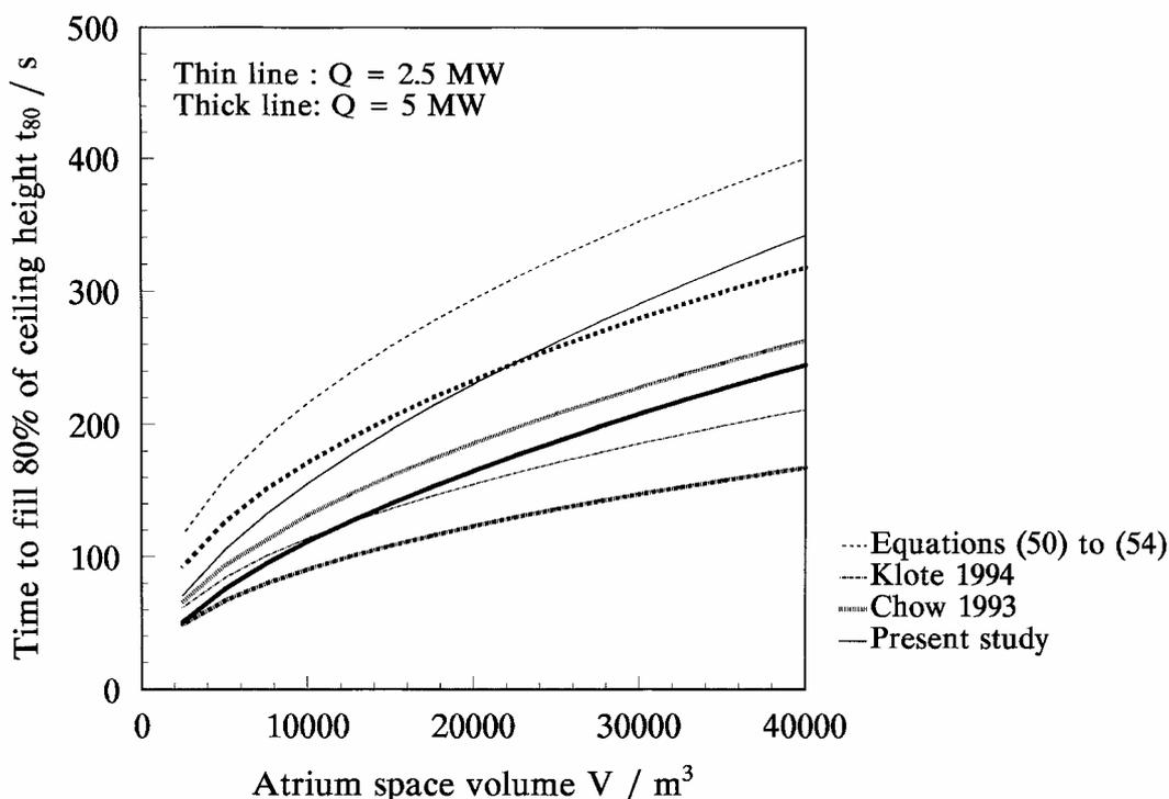
Fig. 6: Time required to fill the smoke layer thickness equal to 80% of the ceiling height
