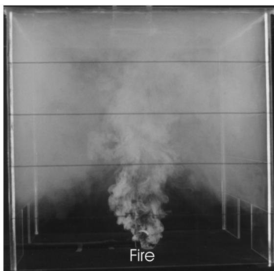
Fig. 2: Typical photograph of the smoke filling process
