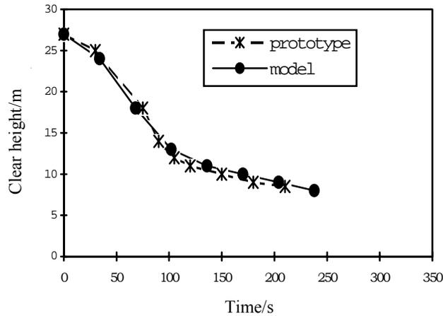
**Fig. 5: Comparison between measured smoke layer height for reduced-scale model and full-scale model prototype**
