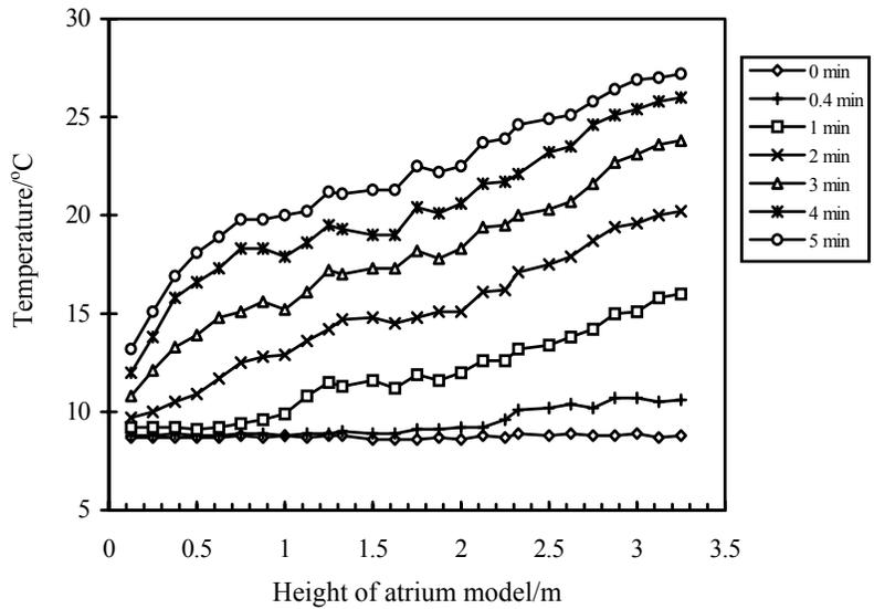
Fig. 3: Vertical temperature distribution versus time
