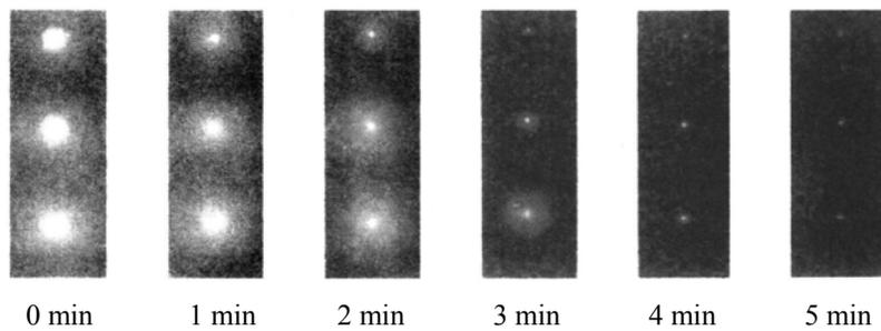
Fig. 4: Distribution of smoke density and visibility versus time
